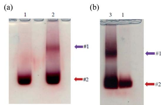
Fig. 9 Agarose electrophoresis of TYMV grafted with AuNP in optimum condition for (a) strategy 1 (lane 2), in comparison with free AuNP (lane 1) and (b) strategy 2 (lane 3). Purple arrow: grafted TYMV. Red arrow: free AuNP.
