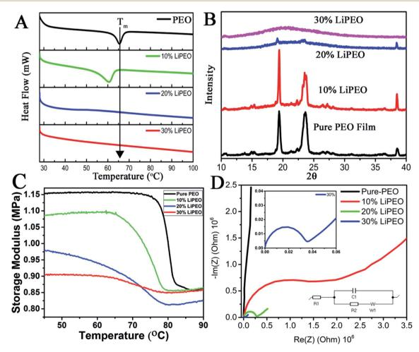
Fig. 1 (A) DSC plots and (B) XRD patterns of different SEs. (C) Storage modulus (MPa) vs. temperature (°C) curves at a frequency of 1 Hz.  ${}^*T_m$  is assigned to the minima of derivative of the sigmoid curves. (D) The EIS (Nyquist plots) of different samples. The simulated Randles circuit which fit the spectra is also shown in the inset.
