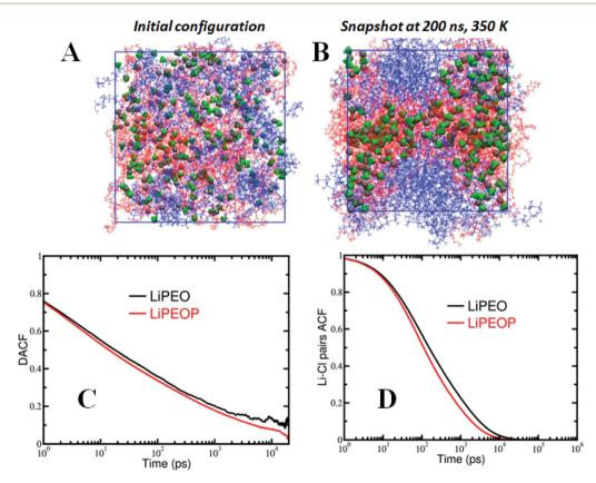
Fig. 4 (A) Initial configuration and (B) equilibrated snapshot at 200 ns of the PEO-PDMS-LiClO<sub>4</sub> electrolyte at 350 K. (C) Dihedral angle autocorrelation function (DACF) of the PEO polymer backbone to understand the effect of PDMS on polymer dynamics, and (D) Li-Cl ion pairs autocorrelation function (ACF).
