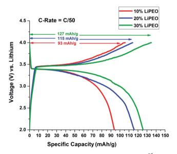
Fig. 3 Effect of salt concentration in PEO electrolyte on 2<sup>nd</sup> cycle of charge discharge of LiFePO<sub>4</sub> half cells at 60 °C.
