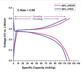
Fig. 6 Charge–discharge cycles showing the effect of addition of PDMS in 20% PEO electrolyte on the  $2^{nd}$  cycle of charge–discharge of LiFePO<sub>4</sub> half cells at 60 °C.
