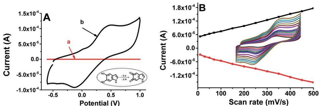
Fig. 3 (A) Cyclic voltammograms of the electrode before (a) and after its modification with Mel-NPs (b) in PBS at 50 mV s<sup>-1</sup>. (B) Plots of anodic and cathodic peak currents vs. scan rates with inset corresponding to CVs of the modified electrode recorded at different scan rates (from inner to outer: 10–500 mV s<sup>-1</sup>).
