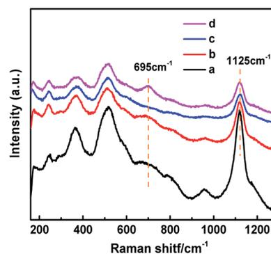
Fig. 6 UV Raman spectra of prepared samples. (a) TS-1; (b) H-TS-1; (c) HCS-TS; (d) HCS-TS<sup>P</sup>.
