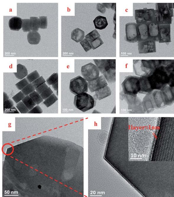
Fig. 2 TEM images of TS-1 (a and d), H-TS-1 (b and e), HCS-TS (TEOS : H-TS-1-80 = 1 : 9) (c and f) and HCS-TS (TEOS : H-TS-1-80 = 0.25 : 9.75) (g and h).
