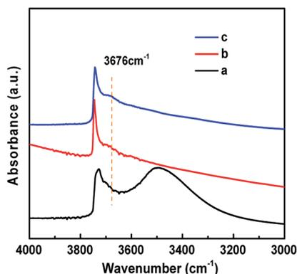
Fig. 4 The FT-IR spectra in the hydroxyl stretching evacuated at 723 K in the range of 1500–4000 cm<sup>-1</sup>. (a) TS-1; (b) H-TS-1; (c) HCS-TS.
