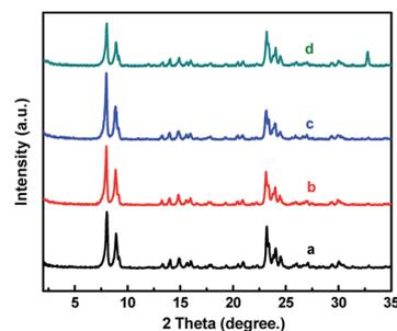
Fig. 1 XRD patterns of the prepared samples. (a) TS-1; (b) H-TS-1; (c) HCS-TS; (d) HCS-TS<sup>P</sup>.
