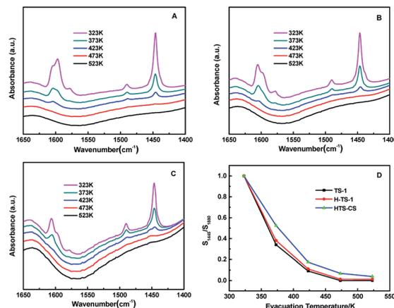
Fig. 5 The FTIR spectra in the pyridine regions of TS-1 (A); H-TS-1 (B); HCS-TS (C) at different evacuation temperatures and the normalized area relative to Lewis acid sites (1445 cm<sup>-1</sup>) vs. evacuation temperatures (D).
