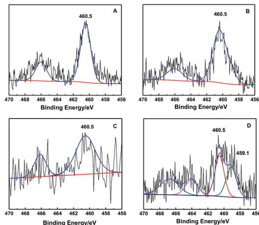
Fig. 7 Ti 2p XPS spectra of TS-1 samples. (A) TS-1, (B) H-TS-1, (C) HCS-TS, (D) HCS-TS<sup>P</sup>.
