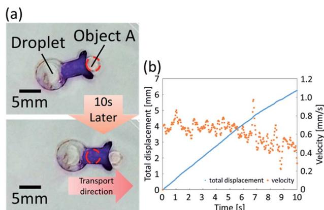
**Fig. 10** (a) Waterborne transport robot. The robot (beetle-shaped exoskeleton + self-propelled droplet) carried object A (red-dyed vegetable oil)  $6.26 \text{ mm}$  in  $10 \text{ s}$ . (b) Displacement and velocity of object A with respect to time. Object A was carried at an average velocity of  $0.61 \text{ mm s}^{-1}$  by the waterborne transport robot.
