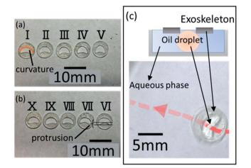
Fig. 5 (a) Exoskeletons with different convex curvatures. (b) Exoskeletons with different concave protrusions. Exoskeleton II and exoskeleton VI have the same boomerang shape. (c) A self-propelled oil droplet fitted with the exoskeleton locomotes in the direction from the concave region toward the convex region. The upper right figure shows a schematic cross-sectional diagram of the experiment.
