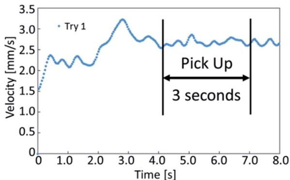
Fig. 3 The graph shows the velocity of a self-propelled droplet. We selected the stable period for 3 seconds while locomoting to determine the average velocity.
