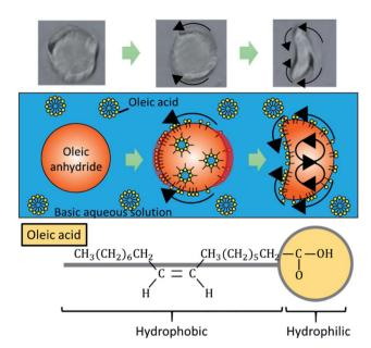
Fig. 1 Self-propulsion mechanism and deformation of oil droplets. The surfactant adheres to the surface of the oil droplet. Marangoni convection occurrs internally due to gradients of surfactant concentration (the darker red areas have higher surface tension). Finally, the droplets transform into the boomerang shape and performed stable straight locomotion.
