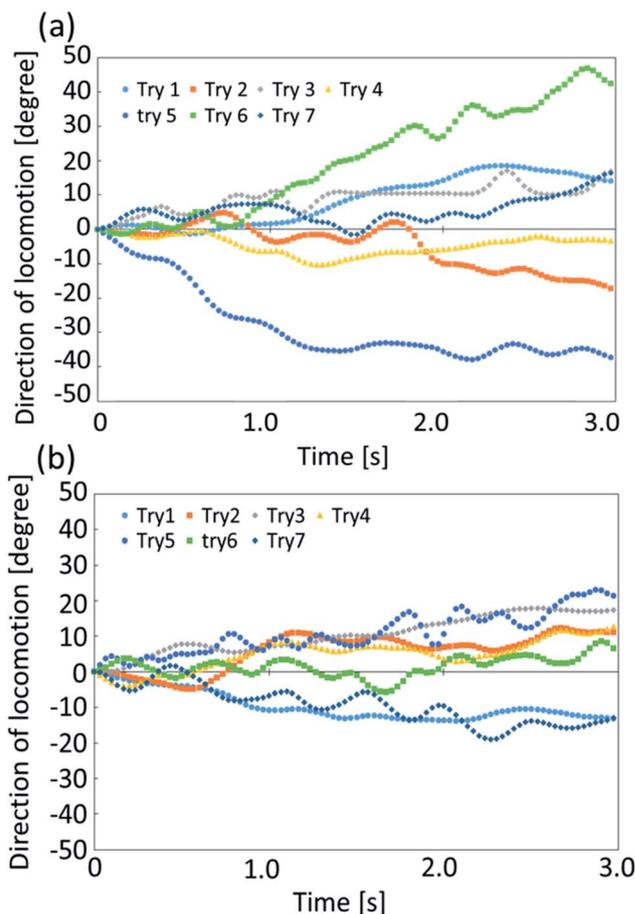
**Fig. 9** Direction of locomotion of the self-propelled oil droplets fitted with exoskeleton IV (a) and X (b) over 3 s, respectively. The direction of locomotion was the summation of angular changes with each moving frame.
