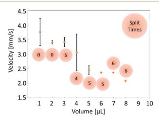
Fig. 4 Comparison of the average velocity for self-propelled oil droplets of different volumes (1–10  $\mu L).$  We conducted 7 experiments for each volume. When the oil droplets split, the trials were excluded from the velocity data. The numbers in the circles indicate the number of times the oil droplets split in 7 experiments. The 1 and 2  $\mu L$  droplets did not split, some of droplets between 3 and 8  $\mu L$  split, and all of the 9 and 10  $\mu L$  droplets split.
