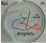
Fig. 2 Locomotion of (a) 2  $\mu L$  and (b) 8  $\mu L$  self-propelled droplets without rigid-frame. Large amount of oil droplets break up into small pieces.
