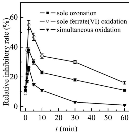
Fig. 2 Toxicity control in the three oxidation systems. (Experimental conditions: TBBPA concentration =  $1.84 \mu\text{mol L}^{-1}$ ; ferrate(VI) concentration =  $0.51 \mu\text{mol L}^{-1}$ ; ozone concentration =  $0.51 \mu\text{mol L}^{-1}$ ; initial solution pH = 7.0; temperature =  $25 \pm 0.5 \text{ }^\circ\text{C}$ ).
