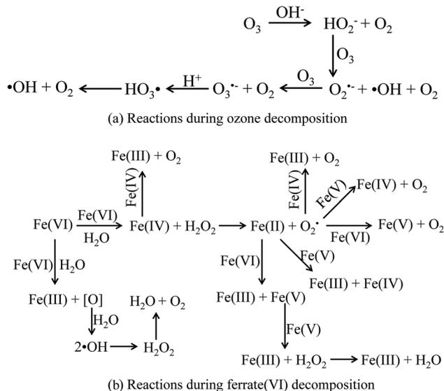
Fig. 7 The decomposition process of ozone and ferrate(vi). (a) Reactions during ozone decomposition; (b) reactions during ferrate(vi) decomposition.
