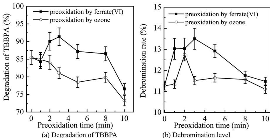
Fig. 3 Optimization of dosing order of oxidants through detection of (a) degradation of TBBPA and (b) debromination level. (Experimental conditions: TBBPA concentration =  $1.84 \mu\text{mol L}^{-1}$ ; ferrate(vi) concentration =  $0.51 \mu\text{mol L}^{-1}$ ; ozone concentration =  $0.51 \mu\text{mol L}^{-1}$ ; initial solution pH = 7.0; temperature =  $25 \pm 0.5 \text{ }^\circ\text{C}$ ).
