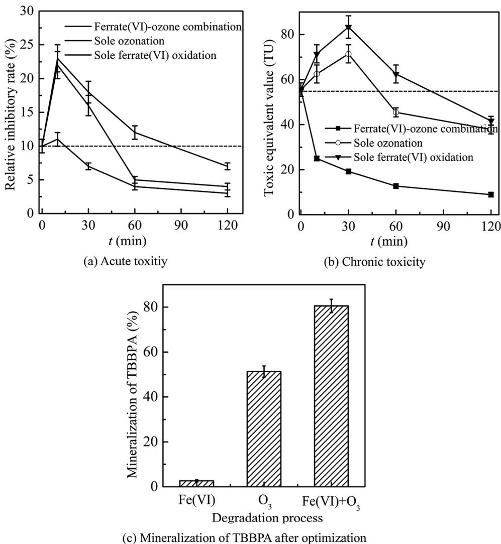
Fig. 6 The control of acute toxicity (a) and the chronic toxicity (b) and mineralization of TBBPA (c) after optimization. (Experimental conditions: TBBPA concentration =  $1.84 \mu\text{mol L}^{-1}$ ; ferrate(vi) concentration =  $0.51 \mu\text{mol L}^{-1}$ ; ozone concentration =  $10.42 \mu\text{mol L}^{-1}$ ; initial solution pH = 7.0; temperature =  $25 \pm 0.5 \text{ }^\circ\text{C}$ ).
