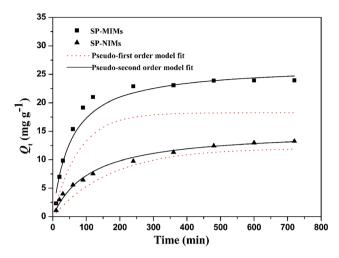
Fig. 5 Kinetic for the adsorption of SP onto SP-MIMs and SP-NIMs under 298 K.
