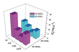
Fig. 6 Selective adsorption capacity of SP-MIMs and SP-NIMs for SP, EM. CHL and AZM.
