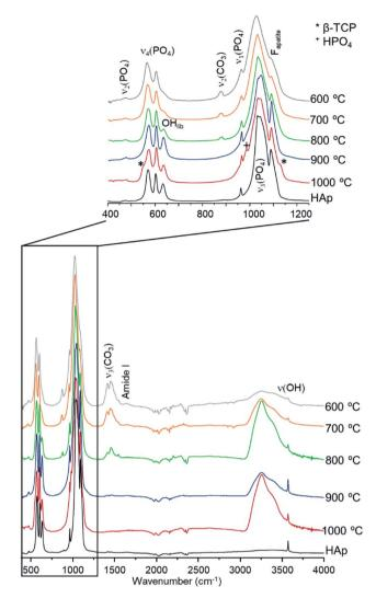
Fig. 3 FTIR-ATR spectra for human tibia (T42) burned from 600 to 1000 °C. (reference hydroxyapatite, HAp, is also shown for comparison.  $F_{apatite}$  refers to fluorapatite. \*Identifies the signals assigned to β-TCP and \*represents the signals assigned to HPO<sub>4</sub>).
