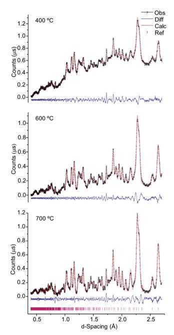
Fig. 4 Refined neutron diffraction data (Hist#5) for human tibial sections (T42) burned at 400, 600 and 700  $^{\circ}$ C.
