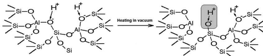
Scheme 2 Schematic drawings of the formation of weak acid sites of H-BEA zeolites.
