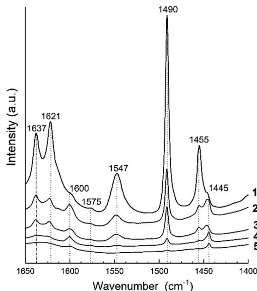
Fig. 5 FTIR spectra of pyridine adsorption for H-BEA zeolites with various Si/Al ratio: (1) H-BEA 15, (2) H-BEA 32, (3) H-BEA 72, (4) H-BEA 124, (5) H-BEA 407.
