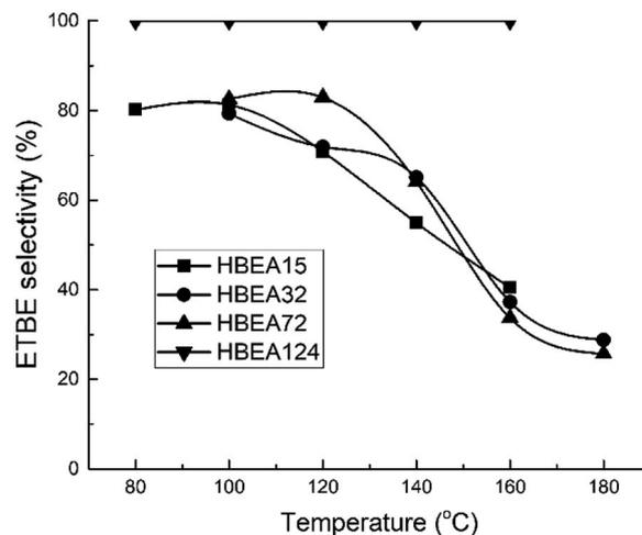
Fig. 10 Temperature dependence of ETBE selectivity for H-BEA zeolites.
