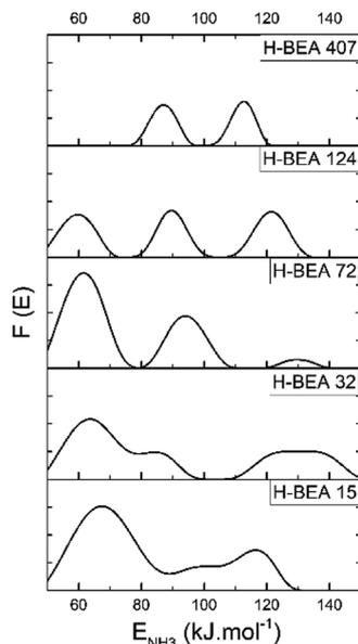
Fig. 4 Ammonia adsorption energy distribution for H-BEA zeolites.
