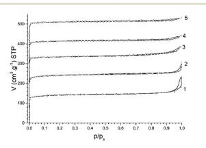
Fig. 2  $N_2$  adsorption isotherms for H-BEA zeolites: (1) H-BEA 15, (2) H-BEA 32, (3) H-BEA 72, (4) H-BEA 124; (5) H-BEA 407.
