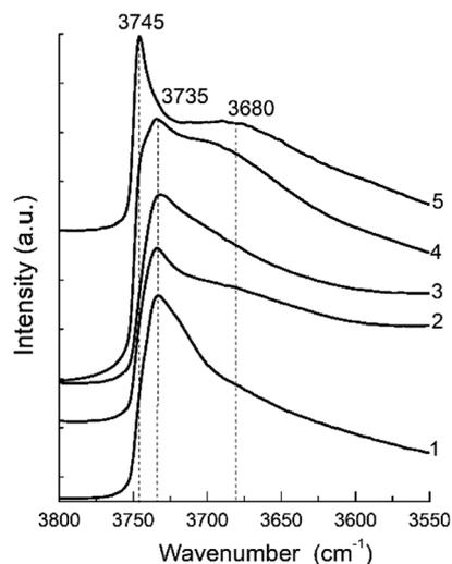
Fig. 7 FTIR spectra of the hydroxyl region of the zeolite H-BEA samples with various Si/Al ratio: (1) H-BEA 15, (2) H-BEA 32, (3) H-BEA 72, (4) H-BEA 124; (5) H-BEA 407.
