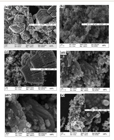
Fig. 2 (a) SEM image of MXene $-\text{Ti}_3\text{C}_2$  material. (b) SEM image of MnO<sub>2</sub> material. (c)-(e) is the MnO<sub>2</sub>/MXene $-\text{Ti}_3\text{C}_2$  nanocomposites with molar ratio 1:2, 1:1 and 2:1 in sequence.
