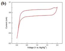
Fig. 4 CV figure of (a) MnO<sub>2</sub> and (b) MnO<sub>2</sub>/MXene-Ti<sub>3</sub>C<sub>2</sub>.
