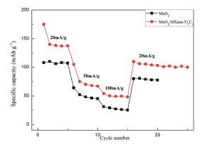
Fig. 5 Rate performance of MnO<sub>2</sub> and MnO<sub>2</sub>/MXene-Ti<sub>3</sub>C<sub>2</sub>.
