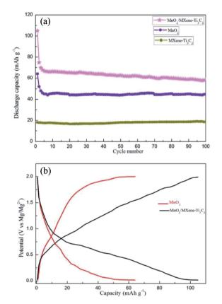
Fig. 3 (a) Cycle performance of MXene $-Ti_3C_2$ , MnO $_2$  and MnO $_2$ /MXene $-Ti_3C_2$  composites with the molar ratio of 1 : 2. (b) Capacity–potential diagram of MnO $_2$  and MnO $_2$ /MXene $-Ti_3C_2$ .
