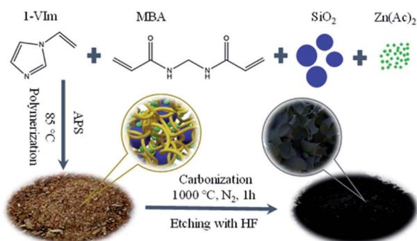
Fig. 1 Schematic illustration of the synthesis of NSHPC.
