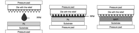
Fig. 1 The scheme of the fabrication of the perovskite thin films using the space-confined conversion of metallic lead with RPM.
