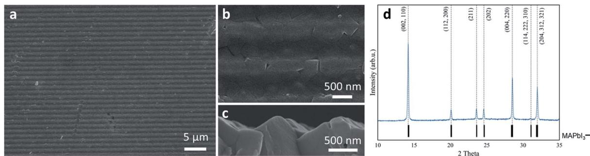
Fig. 2 SEM images (a–c) and XRD (d) of the film obtained by space-confined growth method.
