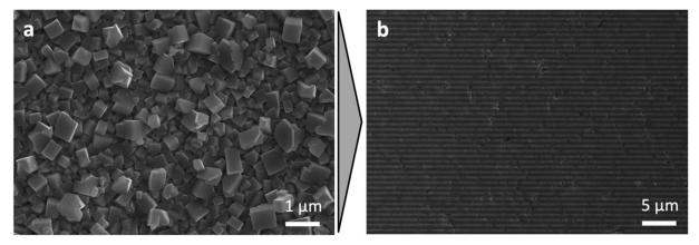
Fig. 3 SEM images of the perovskite film before (a) and after (b) recrystallization in the confined space launched by pressing the die with a relief with a thin layer of RPM on it against that film.
