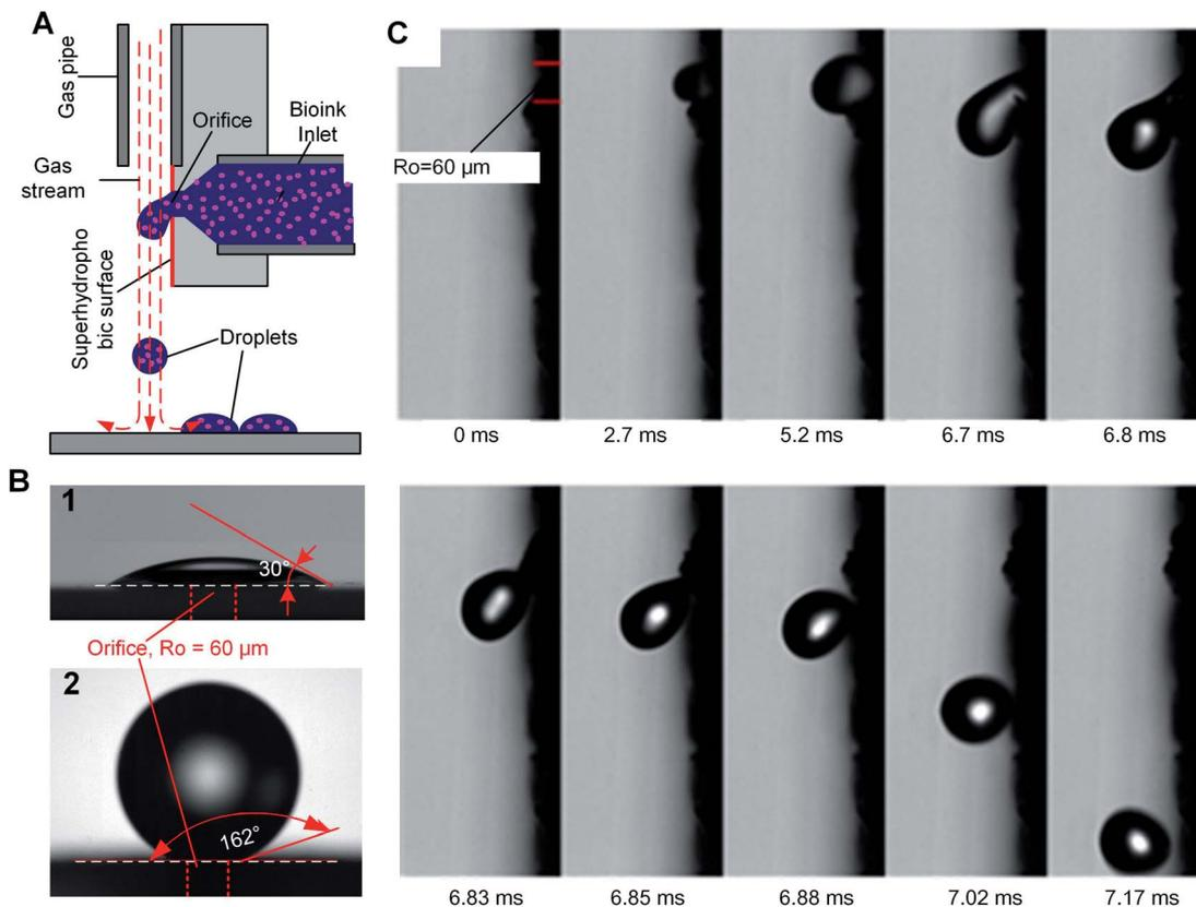
Fig. 1 Pneumatic conveying printing. (A) Principle of PCP; (B) comparison of drops shape on hydrophilic and hydrophobic surface; (C) high speed image of the drop generation and conveying process of PCP.
