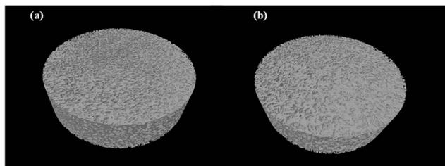
Fig. 6 Micro-CT scan 3D models of composite (a) GO/Na-ALG0.5 and (b) rGO/Na-ALG0.5 scaffolds.
