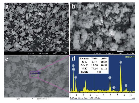
Fig. 3 Morphological and elemental analyses of NPs. (a and b) Low- and high-magnified FESEM images of Mn<sub>2</sub>O<sub>3</sub>/NiO NPs and (c and d) the EDS analysis report.
