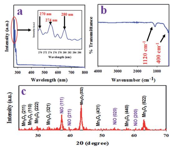
Fig. 2 Optical and structural analysis of the as-synthesized Mn<sub>2</sub>O<sub>3</sub>/NiO NPs. (a) UV-Vis spectrum, (b) FTIR, and (c) X-ray diffraction spectrum of Mn<sub>2</sub>O<sub>3</sub>/NiO NPs.
