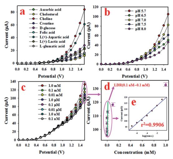
Fig. 4 Optimization and analytical performances of the choline sensor based on the  $Mn_2O_3/NiO$  NP/binder/GCE. (a) Selectivity, (b) pH optimization, (c) electrochemical responses based on the concentration variation of choline from lower to higher, and (d) the calibration curve [inset current vs. log(conc.)].
