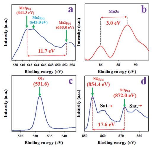
Fig. 1 The XPS analysis of sample  $Mn_2O_3/NiO$  NPs. (a) Core-level XPS of Mn2p, (b) Mn3s orbit, (c) O1s orbit, and (d) high resolution XPS of Ni2p level.
