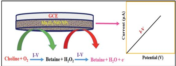
Scheme 1 Pictorial presentation of choline detection in the phosphate buffer medium in electrochemical approaches.
