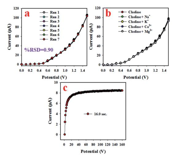
Fig. 5 The reliability performances of the choline sensor based on  $Mn_2O_3/NiO$  NP/binder/GCE. (a) Reproducibility, (b) interference effect of the choline sensor, and (c) the response time.
