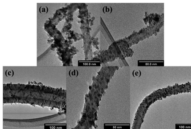
Fig. 7 TEM images of (a) TiO<sub>2</sub>/10% NCNTs, (b) TWZ730/10% NCNTs, (c) TWZ721/10% NCNTs, (d) TWZ712/10% NCNTs and (e) TWZ703/10% NCNTs.
