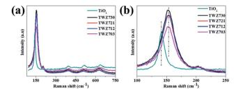
Fig. 2 (a) Laser Raman spectra of  $TiO_2$  and QMMOs and (b) inset showing the  $E_\alpha$  peak.
