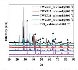
Fig. 5  $\,$  PXRD patterns of  $\rm TiO_2$  and the various QMMOs calcined at 800  $^{\circ}\rm C.$
