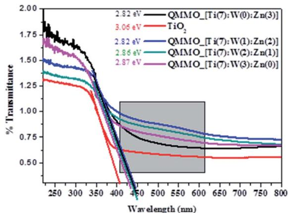
Fig. 6 UV-DRS spectra of TiO<sub>2</sub> and QMMOs.
