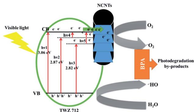
Fig. 9 Proposed BPA photocatalytic mechanism using TWZ721/10% NCNTs.
