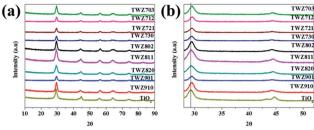
Fig. 1 (a) PXRD patterns of TiO<sub>2</sub> and various QMMOs and (b) inset showing the (101) and (004) reflections of TiO<sub>2</sub> and various QMMOs.
