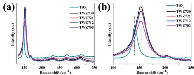
Fig. 2 (a) Laser Raman spectra of TiO<sub>2</sub> and QMMOs and (b) inset showing the E<sub>g</sub> peak.
