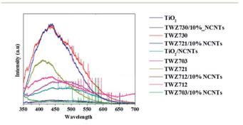
Fig. 8 Photoluminescence emission spectra of  ${\rm TiO_2}$ , QMMO, and composites.
