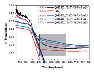
Fig. 6 UV-DRS spectra of TiO<sub>2</sub> and QMMOs
