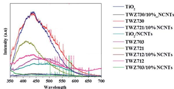
Fig. 8 Photoluminescence emission spectra of TiO<sub>2</sub>, QMМО, and composites.
