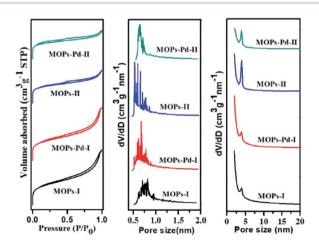
Fig. 3 N<sub>2</sub> adsorption–desorption isotherms and corresponding pore size distributions of MOPs and MOPs-Pd.
