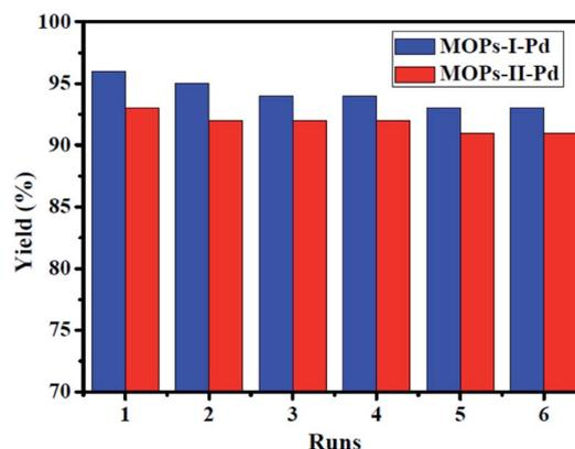
Fig. 7 Recycle test of MOPs-Pd in Heck reaction.
