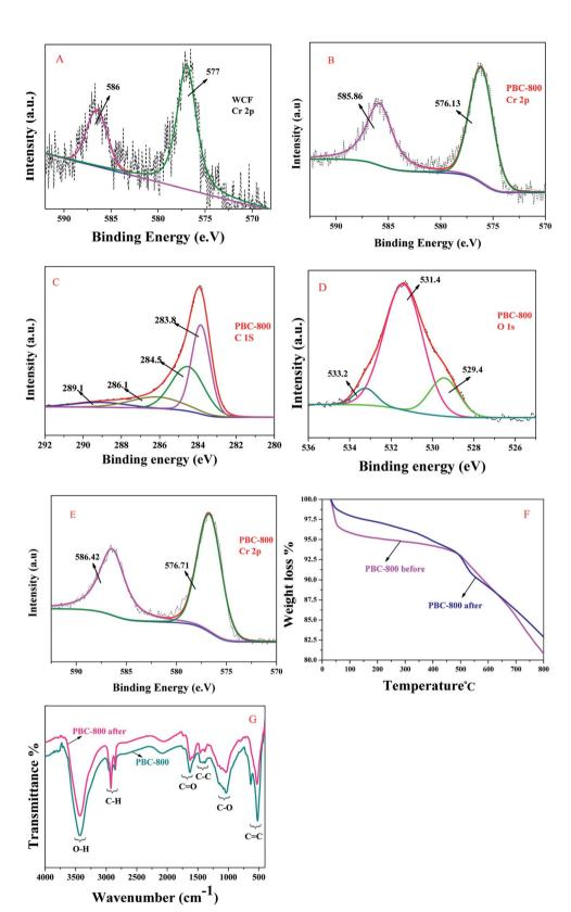
Fig. 6 XPS spectra of WCF (A: Cr 2p) and PBC-800 (B: Cr 2p, C: C 1s, D: O 1s, E: Cr 2p after TC adsorption), thermogravimetric curves (F) and infrared spectra (G) of PBC-800 before and after TC adsorption.
