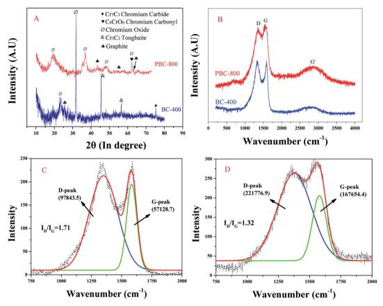
Fig. 1 XRD patterns (A) and Raman spectra (B) of samples. Peak fitting of BC-400 (C) and PBC-800 (D) Raman spectra.
