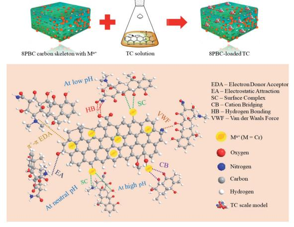
Graphical illustration of the adsorption mechanisms during the adsorption of TC on the PBC-800 surface
