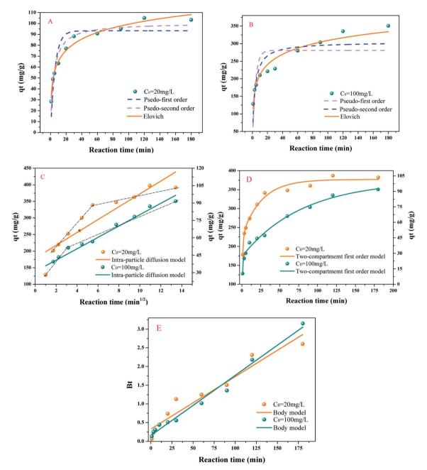
Fig. 3 Kinetic data of TC adsorption on 8PBC (initial concentration is  $20 \text{ mg L}^{-1}$  and  $100 \text{ mg L}^{-1}$ ). Fitting the pseudo-first-order, pseudo-second-order, and Elovich models (A and B), intra-particle diffusion model (C), two-compartment first-order model (D), body model (E).
