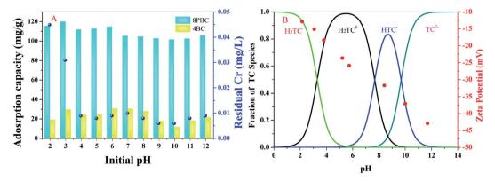
Fig. 4 The effects of initial pH on the adsorption of TC by PBC-800 and BC-400 and the concentration of residual Cr leached after adsorption of TC by PBC-800 at different pH (A), species distribution of TC at different pH and zeta potentials of PBC-800 (B).
