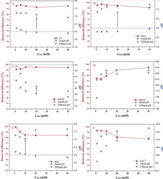
Fig. 5 The effects of coexisting anions (Cl<sup>-</sup>, NO<sub>3</sub><sup>-</sup>, H<sub>2</sub>PO<sub>4</sub><sup>-</sup>, HCO<sub>3</sub><sup>-</sup>, SO<sub>4</sub><sup>2-</sup>, CO<sub>3</sub><sup>2-</sup>) of various concentrations (1, 5, 10, 20, 50 mM) on the adsorption of TC by PBC-800 and pH changes before and after the reaction.
