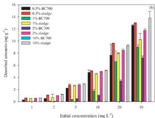
Fig. 2 The adsorption (a) and desorption (b) of carbendazim by BC700 and raw sewage sludge—amended soil at different addition rates.
