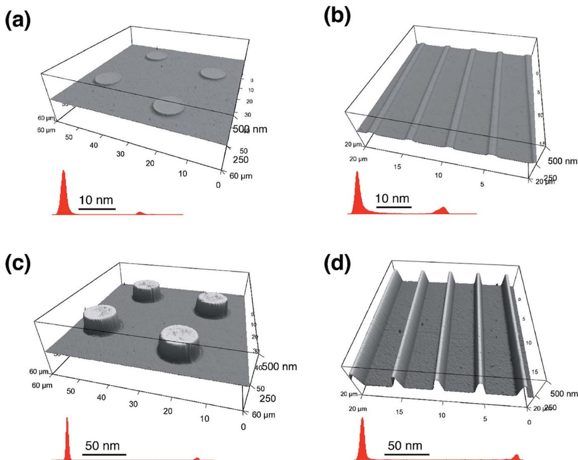
Fig. 8 AFM 3D-topographic images and the corresponding height histogram of TMCTS patterns (a and b) before and (c and d) after VUV/(O)-treatment for 50 min, where (a and c) represent the circular pattern, and (b and d) represent the line pattern.
