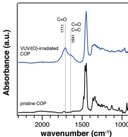
Fig. 2 ATR-FTIR spectra of COP before and after VUV/(O)-irradiation for 10 min.
