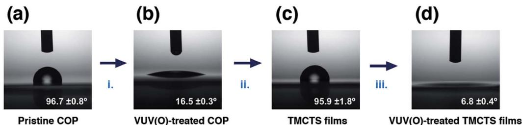
Fig. 6 WCA images and values of (a) pristine COP, (b) VUV/(O)-modified COP, (c) TMCTS thin films and (d) VUV/(O)-treated TMCTS thin films.
