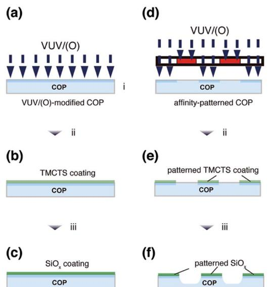
Fig. 1 Schematic illustration of (a) VUV/(O)-modification on COP surface, (b) TMCTS deposition on the modified COP surface, (c)  $\text{SiO}_x$  thin films formed by VUV/(O)-photo-oxidation, (d) affinity-patterning by VUV/(O)-treatment through a photomask, (e) site-selective deposition of TMCTS on the affinity-patterned COP surface, (f)  $\text{SiO}_x$  microstructures on the COP substrate.
