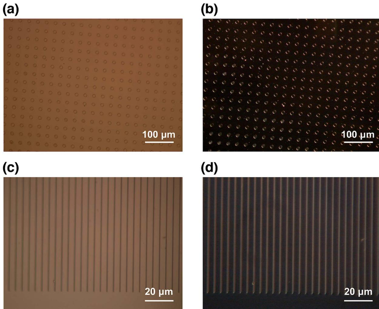
Fig. 9 Optical micrographs of resulting silica micro arrays. The circular patterns with a diameter of 10  $\mu\text{m}$  are shown by (a) bright field image and (b) dark field image. The line patterns with (interval, line width) of (4  $\mu\text{m}$ , 0.5  $\mu\text{m}$ ) are shown by (c) bright field image and (d) dark field image.
