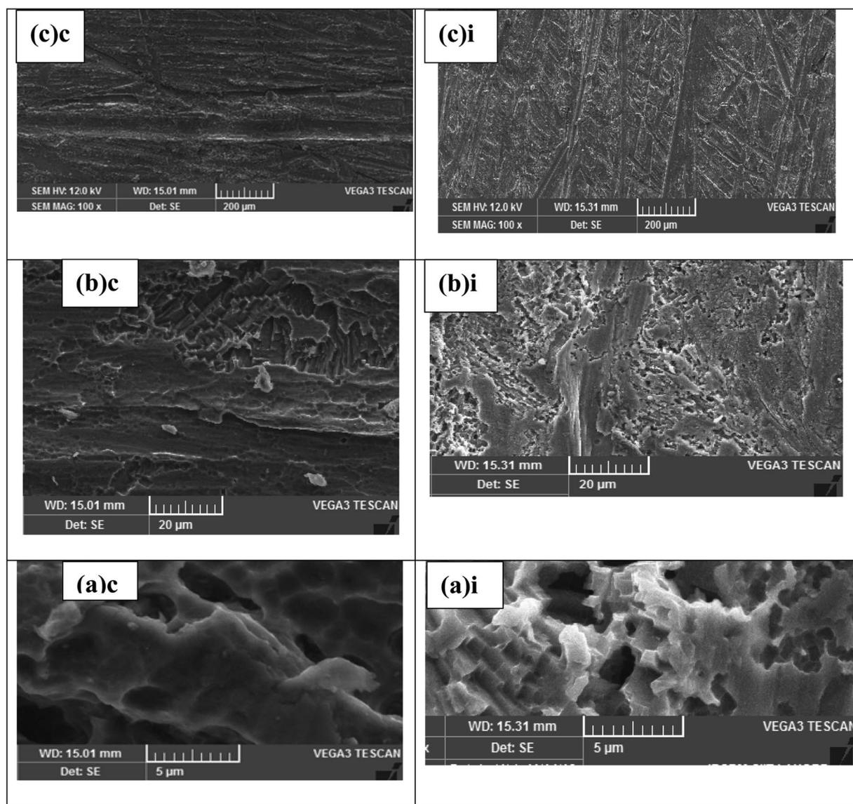
**Fig. 8** SEM micrographs of the aluminum alloy surface without and with UA Schiff base inhibitor: [(a)c] corroded surface at 5 μm, [(a)i] inhibited surface at 5 μm, [(b)c] corroded surface at 20 μm, [(b)i] inhibited surface at 20 μm, [(c)c] corroded surface at 200 μm, [(c)i] inhibited surface at 200 μm.
