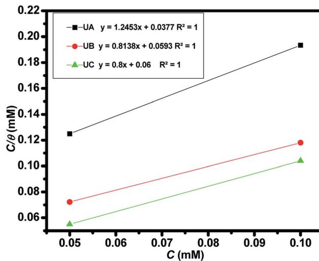
**Fig. 5** Langmuir adsorption isotherm plots for the investigated Schiff base corrosion inhibitors.**Table 4** Adsorption equilibrium constant ( $K_{\text{ads}}$ ) and adsorption free energy ( $\Delta G_{\text{ads}}^\circ$ ) for Schiff bases
