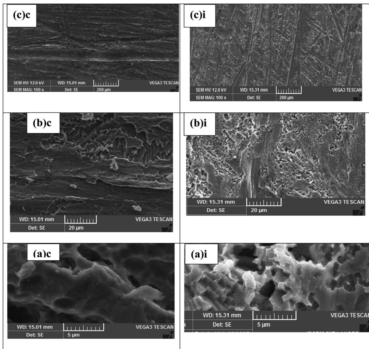
**Fig. 8** SEM micrographs of the aluminum alloy surface without and with UA Schiff base inhibitor: [(a)c] corroded surface at 5  $\mu\text{m}$ , [(a)i] inhibited surface at 5  $\mu\text{m}$ , [(b)c] corroded surface at 20  $\mu\text{m}$ , [(b)i] inhibited surface at 20  $\mu\text{m}$ , [(c)c] corroded surface at 200  $\mu\text{m}$ , [(c)i] inhibited surface at 200  $\mu\text{m}$ .
