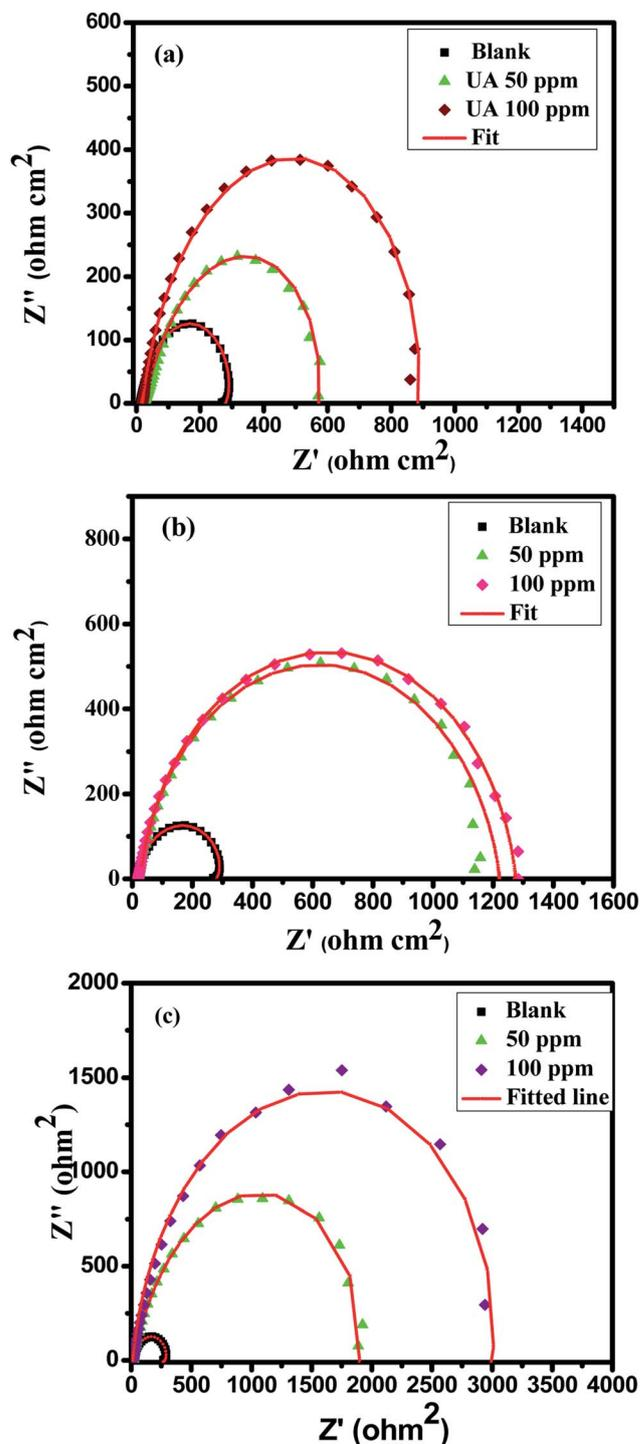
Fig. 2 Nyquist plots for aluminum alloy AA2219-T6 in 0.1 M HCl solution in the absence and presence of Schiff bases (a) **UA**, (b) **UB** and (c) **UC** of 50 and 100 ppm concentrations with their model-fitted overlay.
