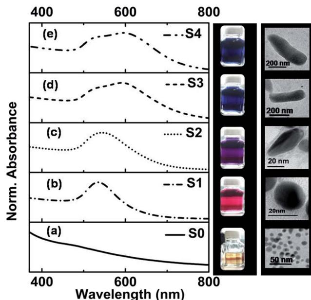
Fig. 1 (a–e) UV-Vis absorption spectra of gold seeds (S0) and the different GNs (S1–S4). The corresponding digital photograph image (color) under visible light illumination and the typical TEM images of the specimens are shown in the adjacent vertical panel (right hand side).
