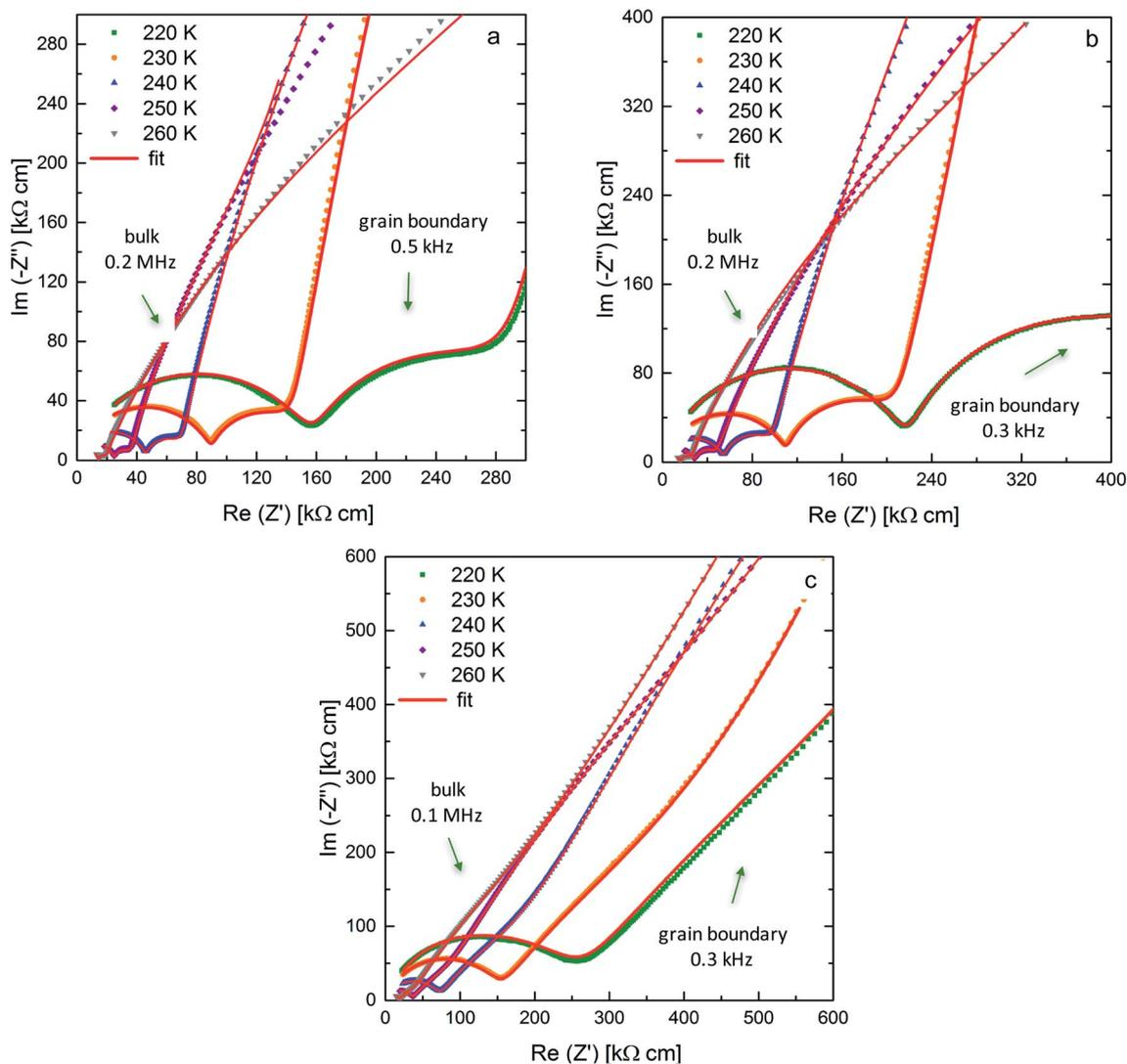
Fig. 3 Nyquist plots and corresponding fits for  $\text{Li}_{7-3x}\text{La}_3\text{Zr}_2\text{Al}_x\text{O}_{12}$  samples ( $x = 0.22$ ) with blocking Au electrodes at 220 K up to 260 K sintered at pressures of 50 MPa (a), 30 MPa (b) and 20 MPa (c).
