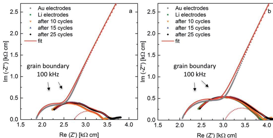
Fig. 7 AC-impedance spectra at 298 K with blocking Au-electrodes and non-blocking Li-electrodes as-prepared and after cycling for samples with  $x = 0.22$ , sintered at 50 MPa (a) and 30 MPa (b).
