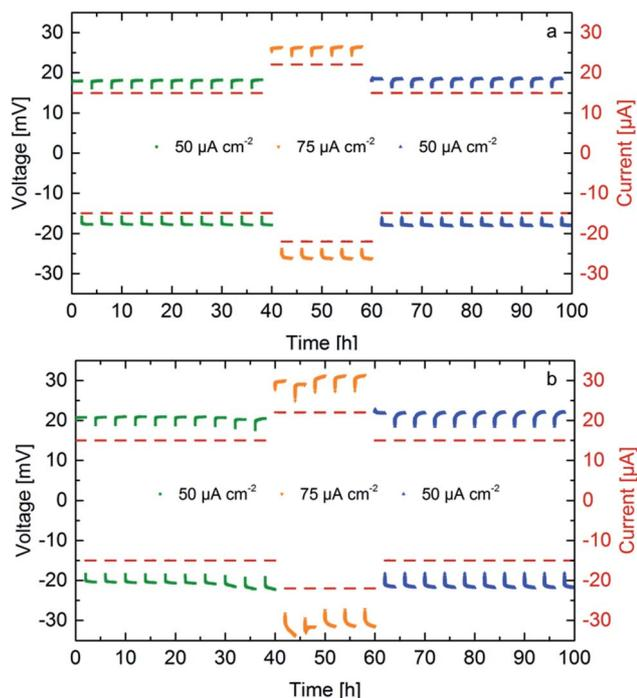
Fig. 6 Galvanostatic cycling of symmetrical cells Li|LLZO|Li at different current densities for  $\text{Li}_{7-3x}\text{La}_3\text{Zr}_2\text{Al}_x\text{O}_{12}$  samples with  $x = 0.22$ , sintered at 50 MPa (a) and 30 MPa (b).
