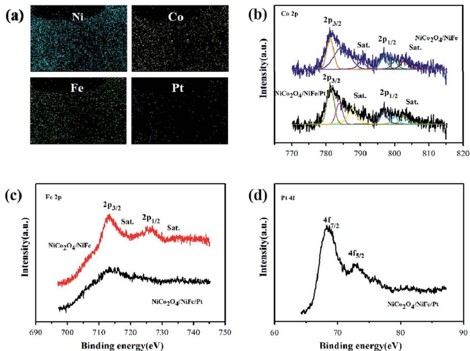
Fig. 5 Elemental mapping images (a). XPS characterization of NiCo<sub>2</sub>O<sub>4</sub>/NiFe and NiCo<sub>2</sub>O<sub>4</sub>/NiFe/Pt hybrid; high-resolution XPS spectra for (b) Co 2p, (c) Fe 2p, and (d) Pt 4f.
