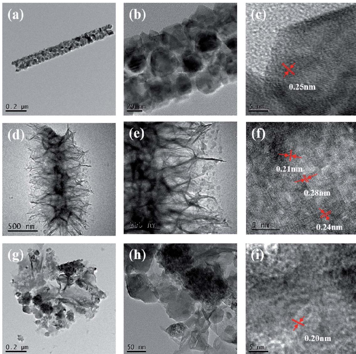
Fig. 4 TEM (a and b) and HRTEM images (c) of the  $\text{NiCo}_2\text{O}_4$  nanowire. TEM (d and e) and HRTEM images (f) of the  $\text{NiCo}_2\text{O}_4/\text{NiFe}$  arrays. TEM (g and h) and HRTEM images (i) of the  $\text{NiCo}_2\text{O}_4/\text{NiFe}/\text{Pt}$  arrays.
