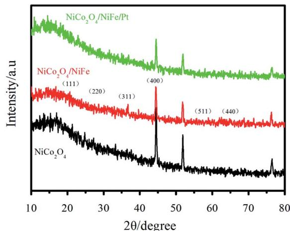
Fig. 2 XRD patterns of the NiCo<sub>2</sub>O<sub>4</sub>, NiCo<sub>2</sub>O<sub>4</sub>/NiFe, and NiCo<sub>2</sub>O<sub>4</sub>/NiFe/Pt nanostructures on NF.
