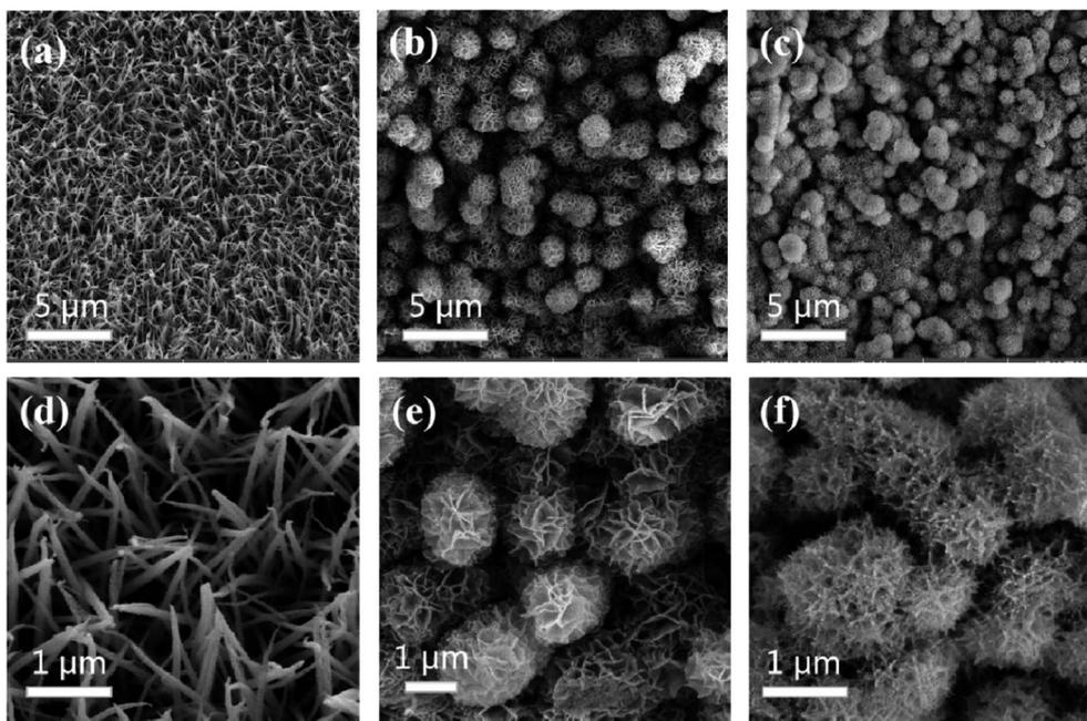
Fig. 3 SEM images of  $\text{NiCo}_2\text{O}_4$  arrays (a and d),  $\text{NiCo}_2\text{O}_4/\text{NiFe}$  arrays (b and e), and  $\text{NiCo}_2\text{O}_4/\text{NiFe}/\text{Pt}$  arrays (c and f) on NF at different magnifications.
