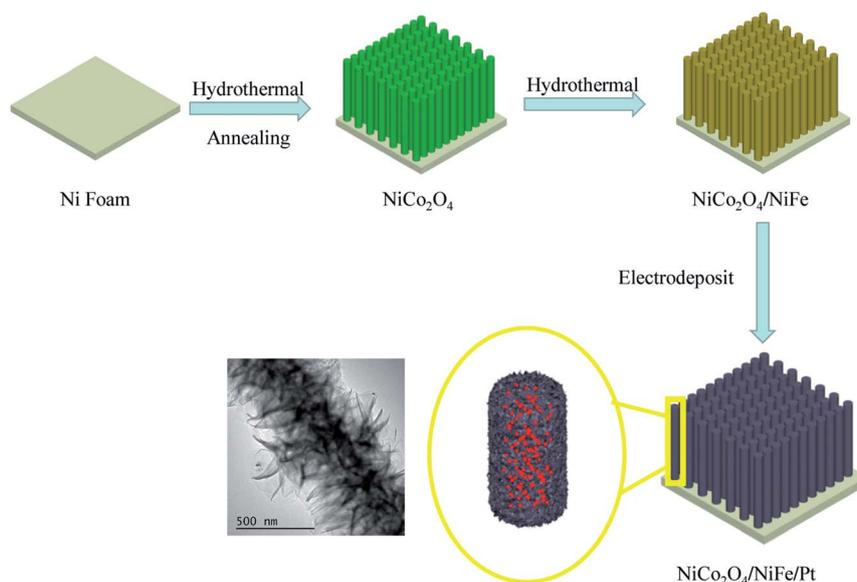
Fig. 1 Schematic of the facile synthesis of NiCo<sub>2</sub>O<sub>4</sub>/NiFe/Pt heterogeneous structure nanowire arrays grown on NF substrate.
