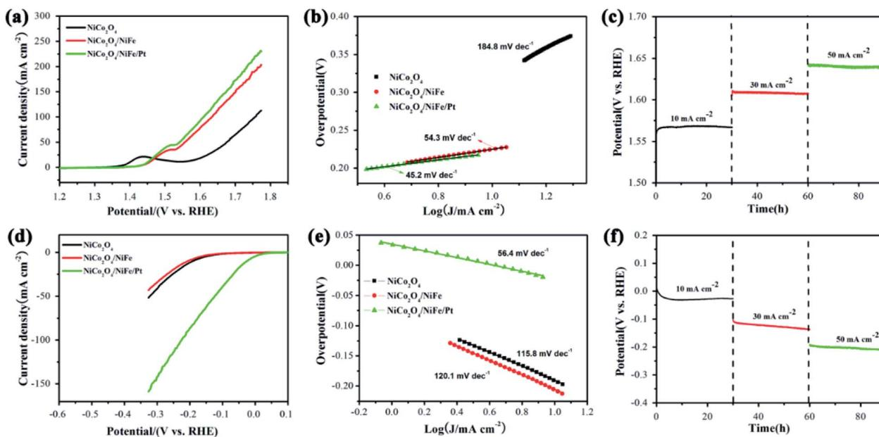
Fig. 6 Bifunctional catalytic performance of NiCo<sub>2</sub>O<sub>4</sub>/NiFe/Pt hybrid electrode on NF in 1.0 M aqueous KOH electrolyte. OER: (a) anodic polarization curves, (b) corresponding Tafel plots, and (c) chronopotentiometry curve. HER: (d) cathodic polarization curves, (e) corresponding Tafel plots, and (f) chronopotentiometry curves.
