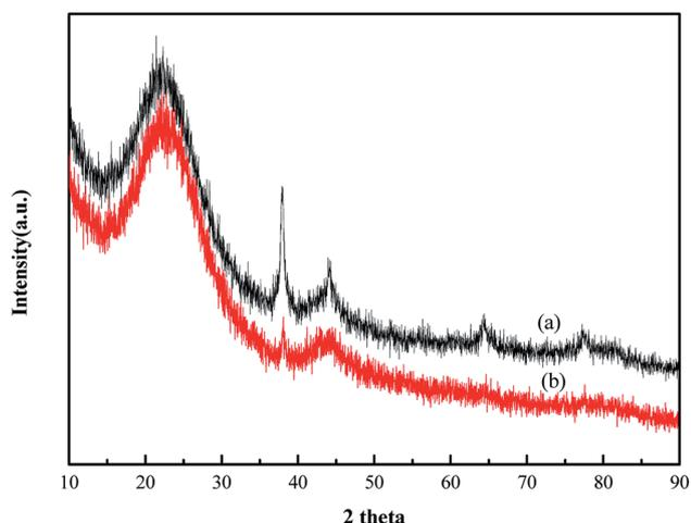
Fig. 2 XRD patterns of the (a) 1% Au/AC and (b) 1% Au/HCS catalysts.
