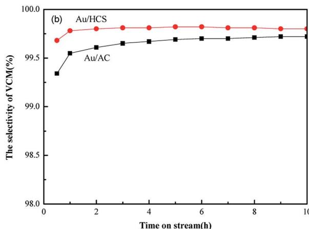
Fig. 5 Conversion of acetylene (a) and selectivity of VCM (b) in acetylene hydrochlorination catalyzed by the Au/HCS and Au/AC catalysts (GHSV =  $870 \text{ h}^{-1}$ ,  $V_{\text{HCl}}/V_{\text{C}_2\text{H}_2} = 1.15$ , reaction temperature =  $180 \text{ }^\circ\text{C}$ ).
