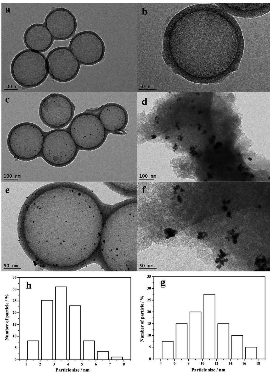
Fig. 3 TEM data on the (a and b) HCS, (c and e) Au/HCS, (d and f) Au/AC. The figure also shows the catalysts and particle size histograms of (g) Au/HCS and (h) Au/C catalysts.
