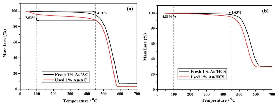
Fig. 8 TGA curves of (a) Au/AC and (b) Au/HCS catalysts.
