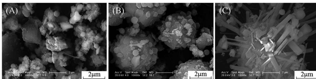
Fig. 5 SEM images of MPs-6 prepared at (A) 0.2, (B) 2 and (C) 4 h.
