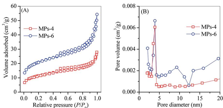
Fig. 10  $N_2$  adsorption isotherms (A) and pore volume (B) of MPs-4 and MPs-6.
