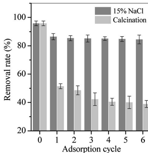
Fig. 11 Adsorption capacity of MPs-6 regenerated with 15% NaCl solution and calcination at  $450 \text{ }^\circ\text{C}$  for 2 h (adsorption condition: initial pH = 5, equilibrium time = 48 h and initial volume = 20 mL).
