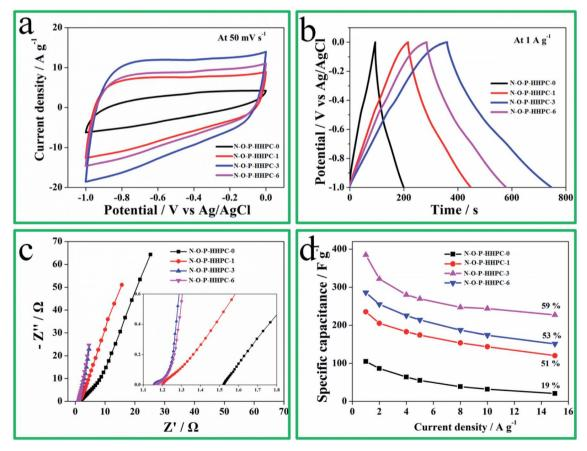
Fig. 4 The electrochemical performances of N-O-P-HHPC-0, N-O-P-HHPC-1, N-O-P-HHPC-3 and N-O-P-HHPC-6 tested in 6 KOH using the three electrode system. (a) CV curves at 50 mV s<sup>-1</sup>. (b) GCD curves at 1 A g<sup>-1</sup>. (c) EIS curves, the inset at lower right corner is the zoom-in Nyquist plots. (d) The specific capacitances at different current densities.
