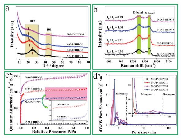
Fig. 2 XRD patterns (a), Raman spectra (b),  $N_2$ -adsorption and desorption isotherms (c) and pore size distributions (d) of N-O-P-HHPC-0, N-O-P-HHPC-1, N-O-P-HHPC-3 and N-O-P-HHPC-6.
