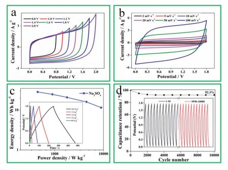
Fig. 5 The electrochemical performances of N-O-P-HHPC-3//N-O-P-HHPC-3 symmetrical SCs using 1 M  $Na_2SO_4$  gel electrolyte. (a) CV curves of different potential windows at 10 mV s<sup>-1</sup>. (b) CV curves of different scan rates. (c) Ragone plot, inset of (c) is GCD curves at different current densities. (d) Cycling stability efficiency at 10 A g<sup>-1</sup>, inset of (d) is the first 10 cycles and the last 10 cycles.
