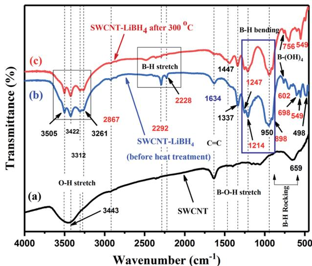
Fig. 2 FTIR spectra of (a) pristine SWCNT, (b) SWCNT-LiBH<sub>4</sub> composite (before heat treatment) and (c) SWCNT-LiBH<sub>4</sub> composite heat treated at 300 °C in air (SWLiB-A).
