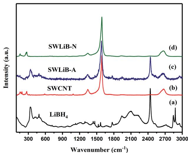
Fig. 3 Raman spectra of (a) LiBH<sub>4</sub>, (b) pristine SWCNT, (c) SWCNT-LiBH<sub>4</sub> composite treated at 300 °C under air (SWLiB-A) and (d) SWCNT-LiBH<sub>4</sub> composite treated at 500 °C under nitrogen (SWLiB-N).
