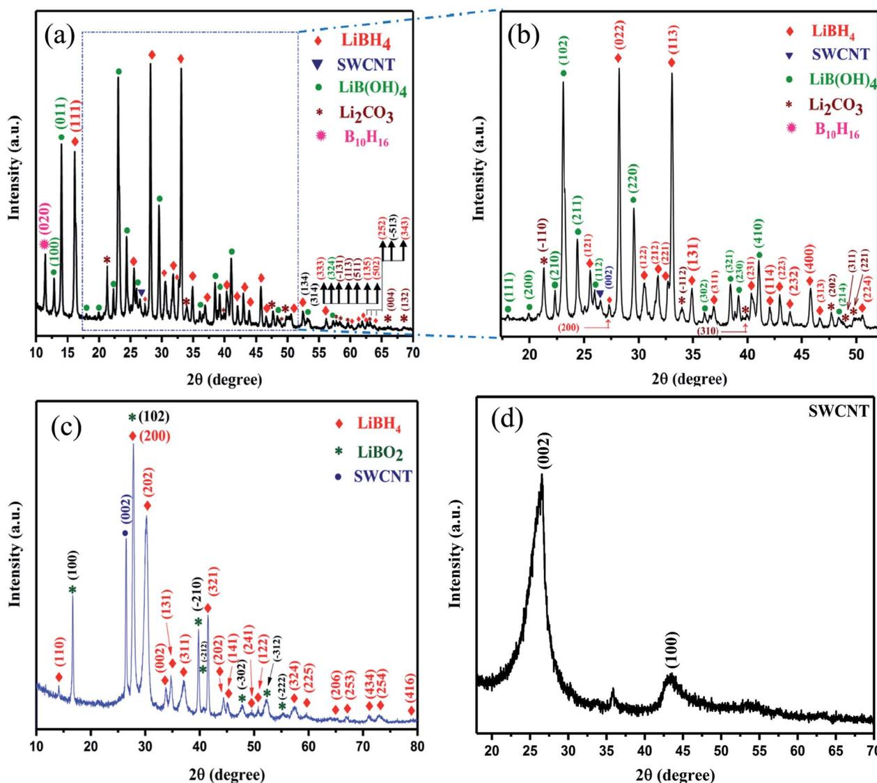
Fig. 1 XRD pattern of (a) SWCNT–LiBH<sub>4</sub> composites treated at 300 °C under air (SWLiB-A), (b) enlarged XRD pattern of SWLiB-A in the range of 2θ = 15–52°, (c) SWCNT–LiBH<sub>4</sub> treated at 500 °C under nitrogen environment (SWLiB-N) and (d) pristine SWCNT.
