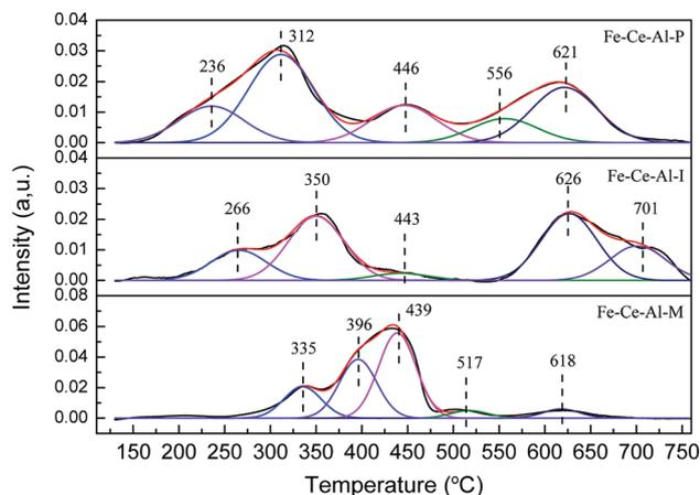
Fig. 5 H<sub>2</sub>-TPR profiles of different catalysts.
