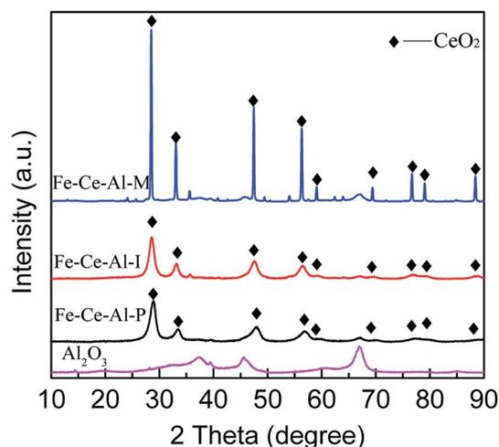
Fig. 2 XRD patterns of different Fe–Ce–Al catalysts and Al<sub>2</sub>O<sub>3</sub> support.
