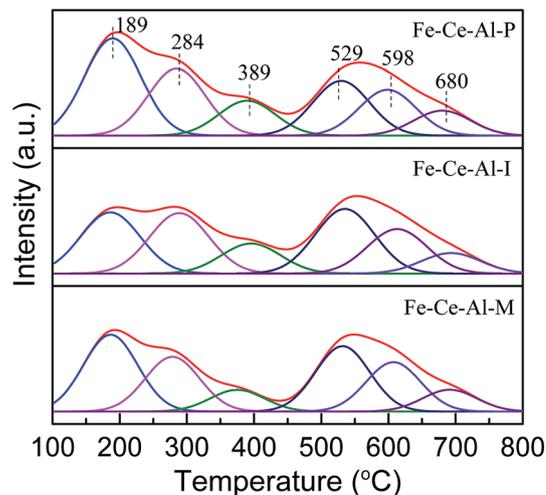
Fig. 4  $NH_3$ -TPD profiles of different catalysts.
