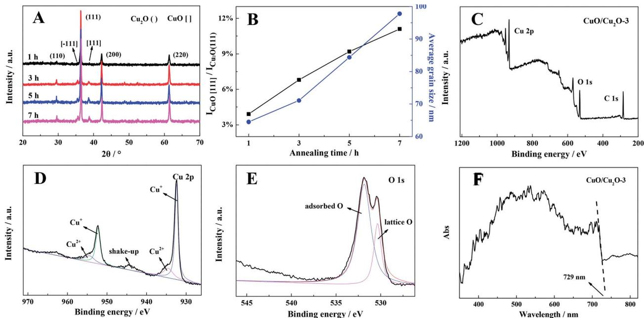
Fig. 1 (A) XRD patterns of different samples; (B) the variations in  $I_{\text{CuO}(111)}/I_{\text{Cu}_2\text{O}(111)}$  and average grain sizes influenced by annealing time over different samples; (C) XPS spectra of the CuO/Cu<sub>2</sub>O-3 composite, (D) Cu2p, and (E) O1s; and (F) UV-Vis DRS spectrum of the CuO/Cu<sub>2</sub>O-3 composite.
