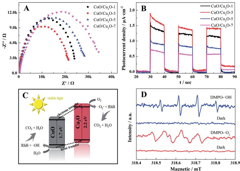
Fig. 4 (A) Electrochemical impedance spectra and (B) transient photocurrent responses of different samples; (C) possible photocatalytic reaction mechanism of the CuO/Cu<sub>2</sub>O-3 composite; (D) DMPO spin-trapping ESR spectra of the CuO/Cu<sub>2</sub>O-3 composite in methanol and water for ·O<sub>2</sub><sup>-</sup> and ·OH before and after 10 min illumination, respectively.
