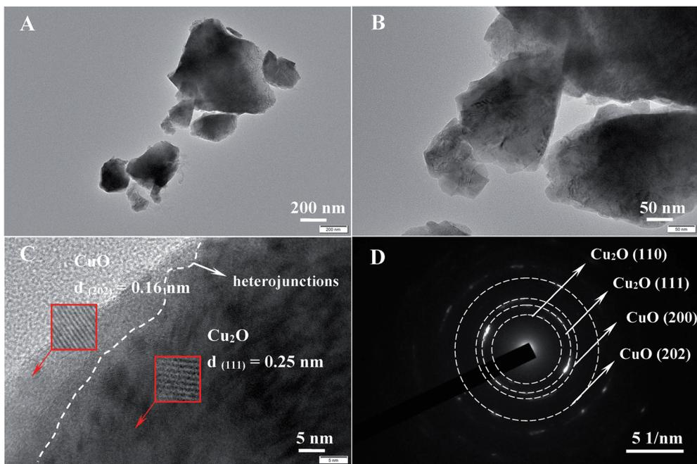
Fig. 2 (A–C) TEM images and (D) SAED pattern of the CuO/Cu<sub>2</sub>O-3 sample.
