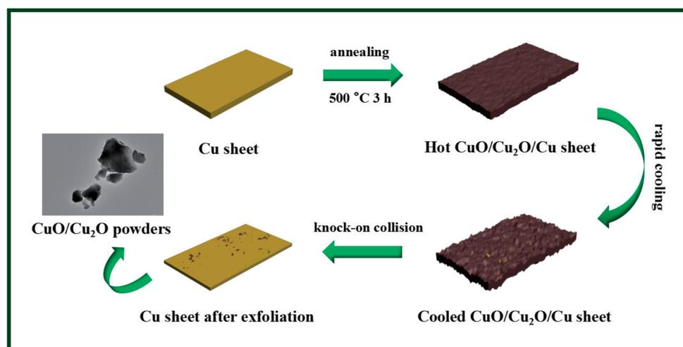
Scheme 1 The CuO/Cu<sub>2</sub>O composites were synthesized *via* a facile one-step thermal exfoliation process from a commercial copper sheet.
