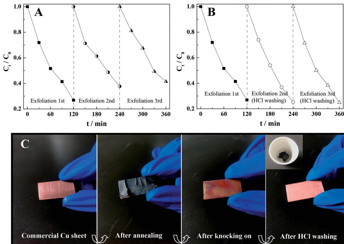
Fig. 5 (A) Stability test results of  $\text{CuO}/\text{Cu}_2\text{O}$ -3 for cycled thermal exfoliation under visible light irradiation; (B) stability test results of  $\text{CuO}/\text{Cu}_2\text{O}$ -3 for cycled thermal exfoliation after HCl washing under the same conditions; and (C) schematic of the fabrication procedure towards the  $\text{CuO}/\text{Cu}_2\text{O}$  nanocomposite powders.
