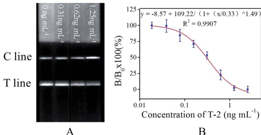
Fig. 3 (A) Photo of ICA strips with different concentrations of T-2 under 365 nm UV excitation by gel imager. (B) Standard inhibition curve for T-2 was obtained by plotting the normalized signal  $B/B_0 \times 100\%$  against the logarithm of T-2 concentration. Data were carried out in triplicate.
