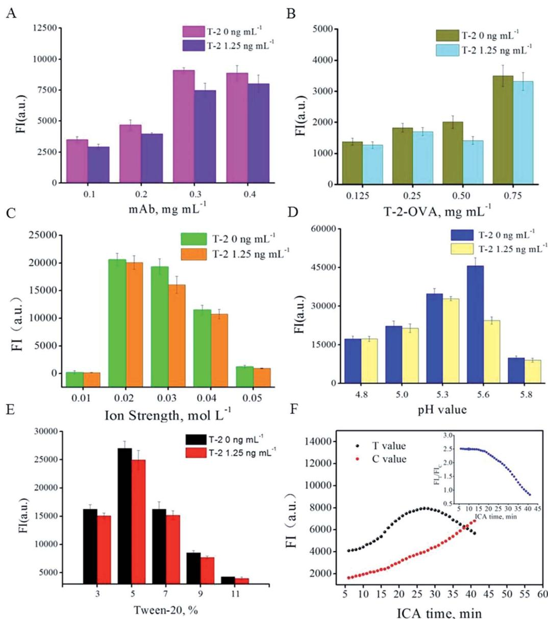
Fig. 2 (A) Estimation of the optimal labeling amount of anti-T-2-mAb on QBs. (B) Optimization of T-2-OVA concentration on the T line. (C) Effect of ion strength on FI. (D) Effect of pH value on FI. (E) Optimization of optimal Tween-20 concentration in the ICA system. (F) Immuno-reaction dynamics of  $FI_T$ ,  $FI_C$ , and  $FI_T/FI_C$  (inset). Optimization from A to E were carried out in competitive inhibition mode with T-2 spiked concentration of 0 and 1.25 ng mL<sup>-1</sup>.
