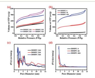
Fig. 2 BET adsorption isotherm for DDHPC 1kh, 2kh, 3kh and 4kh (a), and DDHPC-4, 4k and 4hk (b); pore size distribution for DDHPC-1kh, 2kh and 3kh (c), and DDHPC-4, 4k and 4hk (d).
