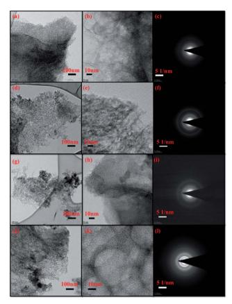
Fig. 4 TEM image of different DDHPC-kh samples; DDHPC-1kh (a-c), DDHPC-2kh (d-f), DDHPC-3kh (g-i), DDHPC-4kh (j-l)
