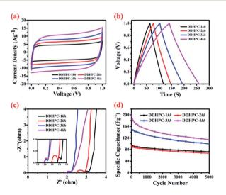
Fig. 5 Comparative electrochemical data for DDHPC 1kh, 2kh, 3kh and 4kh samples; (a) cyclic voltammetry (scan rate 100 mV s<sup>-1</sup>), (b) chronopotentiometry charge-discharge (current density 1 A  $g^{-1}$ ), (c) Nyquist plot for impedance and (d) cyclic stability at current density of  $10 \text{ A g}^{-1}$ .
