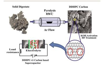
**Scheme 1** Schematic diagram for the synthesis of DDHPC-kh carbon from anaerobic digestate.
