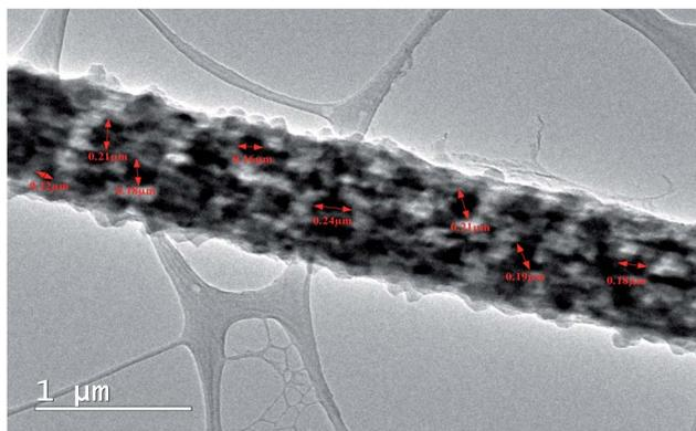
Fig. 5 TEM micrograph of single DIPAB–PVDF (DIPAB 5%) nanofiber incorporated with nanoparticles of DIPAB.
