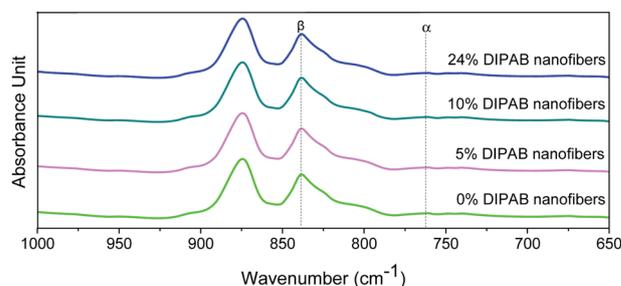
**Fig. 3** FTIR spectra of DIPAB–PVDF composite films for varying weight ratios 0–24% showing the formation of the dominating electroactive  $\beta$ -phase in electrospun nanofibers.
