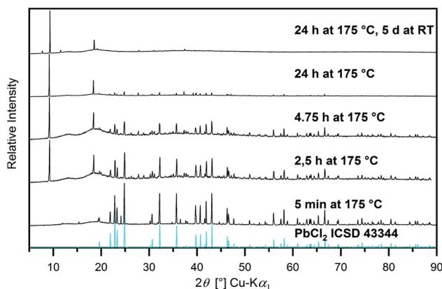
Fig. 10 PXRD patterns of the sample PbO + [Hbet][NTf<sub>2</sub>] + [Hbet]Cl ( $n_{\text{Pb}} : n_{[\text{Hbet}][\text{NTf}_2]} : n_{[\text{Hbet}]\text{Cl}} = 1 : 4 : 2$ ) after different reaction times compared to the diffractogram of PbCl<sub>2</sub> simulated from single crystal data (blue) in the range  $5^\circ \leq 2\theta \leq 90^\circ$ .
