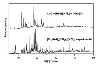
Fig. 9 Experimental diffractogram of the sample CuO + [Hbet][NTf<sub>2</sub>] + [Hbet]Cl (4 h reaction time, top) compared to the experimental diffractogram of  $[Cu_2(bet)_4(NTf_2)_2][NTf_2]_2$  in the range  $5^{\circ} \le 2\theta \le 90^{\circ}$ .
