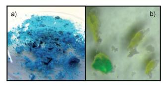
Fig. 5 Images of (a)  $[Cu_2(bet)_4(NTf_2)_2][NTf_2]_2$  and (b) the discolouration in  $[P_{66614}]Cl$  accompanied by the yellowing of the surrounding IL.
