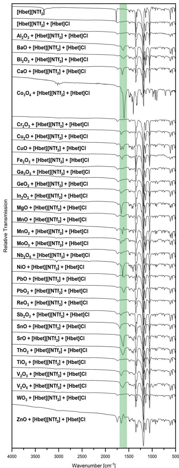
Fig. 8 IR spectra of [Hbet][NTf<sub>2</sub>], [Hbet]<sub>2</sub>[NTf<sub>2</sub>]Cl and all samples of a metal oxide in [Hbet]<sub>2</sub>[NTf<sub>2</sub>]Cl stirred at 175 °C for 24 h in the range of 500 cm<sup>-1</sup> ≤ ν̄ ≤ 4000 cm<sup>-1</sup>. The range of a bands attributed to ν<sub>as</sub> COO of a coordinated betaine carboxylate group is highlighted in green.
