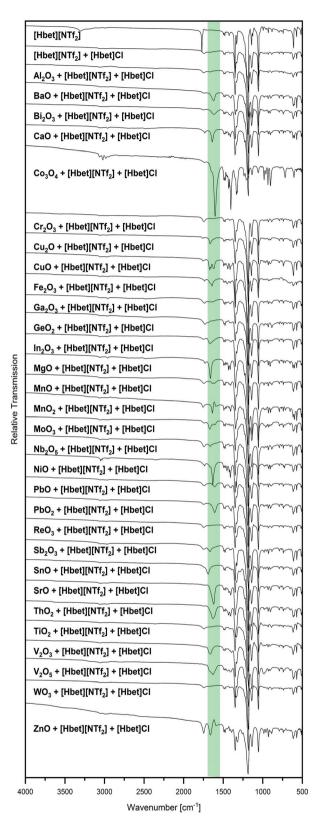
Fig. 8 IR spectra of [Hbet][NTf<sub>2</sub>], [Hbet]<sub>2</sub>[NTf<sub>2</sub>]Cl and all samples of a metal oxide in [Hbet]<sub>2</sub>[NTf<sub>2</sub>]Cl stirred at 175 °C for 24 h in the range of 500 cm<sup>-1</sup>  $\leq \tilde{\nu} \leq$  4000 cm<sup>-1</sup>. The range of a bands attributed to  $\nu_{as}$ COO of a coordinated betaine carboxylate group is highlighted in areen
