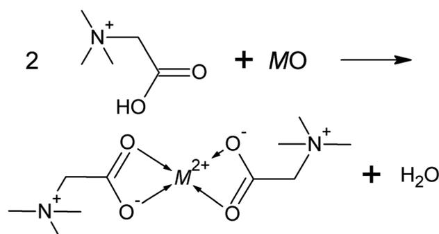
Fig. 1 Schematic reaction of a metal oxide and [Hbet][NTf<sub>2</sub>] resulting in a coordination compound and water (M<sup>2+</sup> = metal ion).
