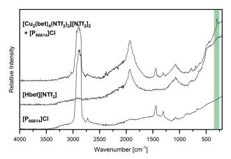
Fig. 7 Raman spectrum of [Cu<sub>2</sub>(bet)<sub>4</sub>(NTf<sub>2</sub>)<sub>2</sub>][NTf<sub>2</sub>]<sub>2</sub> that was stirred at 60 °C in [P<sub>66614</sub>]Cl for 19 h (top) compared to the spectra of [Hbet] [NTf<sub>2</sub>] (middle) and [P<sub>66614</sub>]Cl (bottom) in the range 200 cm<sup>-1</sup>  $\leq \tilde{v} \leq$  $4000 \text{ cm}^{-1}$ . The position of  $v_s$  CuCl is highlighted in green.
