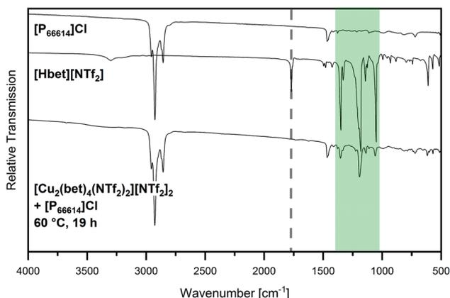
Fig. 6 IR spectrum of  $[Cu_2(bet)_4(NTf_2)_2][NTf_2]_2$  that was stirred at  $60\text{ }^\circ\text{C}$  in  $[P_{66614}]Cl$  for 19 h (bottom) compared to the spectra of  $[Hbet][NTf_2]$  (middle) and  $[P_{66614}]Cl$  (top) in the range  $500\text{ cm}^{-1} \leq \tilde{\nu} \leq 4000\text{ cm}^{-1}$ . The position of  $\nu_{as} COO$  of  $[Hbet]^+$  is marked with a dotted line and the region of the most intensive bands of  $[Hbet][NTf_2]$  is highlighted in green.
