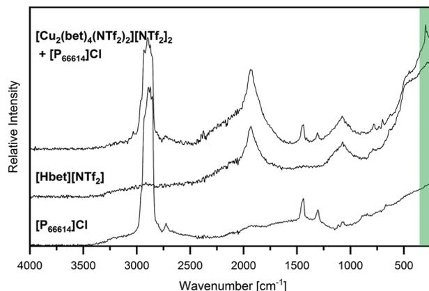
Fig. 7 Raman spectrum of  $[Cu_2(bet)_4(NTf_2)_2][NTf_2]_2$  that was stirred at  $60\text{ }^\circ\text{C}$  in  $[P_{66614}]Cl$  for 19 h (top) compared to the spectra of  $[Hbet][NTf_2]$  (middle) and  $[P_{66614}]Cl$  (bottom) in the range  $200\text{ cm}^{-1} \leq \tilde{\nu} \leq 4000\text{ cm}^{-1}$ . The position of  $\nu_s CuCl$  is highlighted in green.
