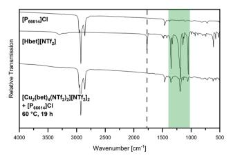
Fig. 6 IR spectrum of  $[Cu_2(bet)_4(NTf_2)_2][NTf_2]_2$  that was stirred at 60 °C in [P<sub>66614</sub>]Cl for 19 h (bottom) compared to the spectra of [Hbet] [NTf<sub>2</sub>] (middle) and [P<sub>66614</sub>]Cl (top) in the range 500 cm<sup>-1</sup>  $\leq \tilde{\nu} \leq$ 4000 cm<sup>-1</sup>. The position of  $v_{as}$  COO of [Hbet]<sup>+</sup> is marked with a dotted line and the region of the most intensive bands of [Hbet][NTf2] is highlighted in green.
