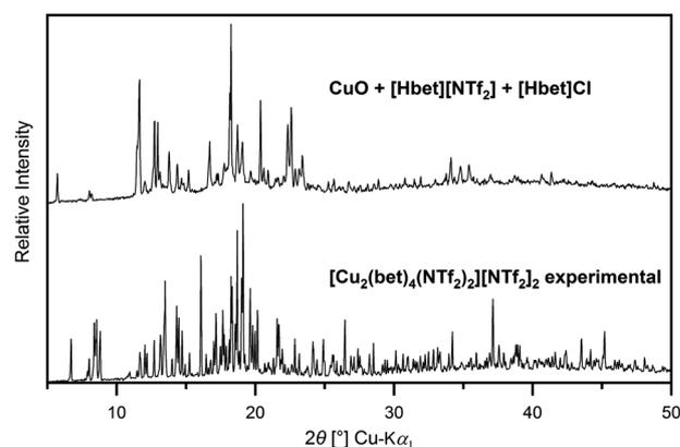
Fig. 9 Experimental diffractogram of the sample CuO + [Hbet][NTf<sub>2</sub>] + [Hbet]Cl (4 h reaction time, top) compared to the experimental diffractogram of [Cu<sub>2</sub>(bet)<sub>4</sub>(NTf<sub>2</sub>)<sub>2</sub>][NTf<sub>2</sub>]<sub>2</sub> in the range 5° ≤ 2θ ≤ 90°.
