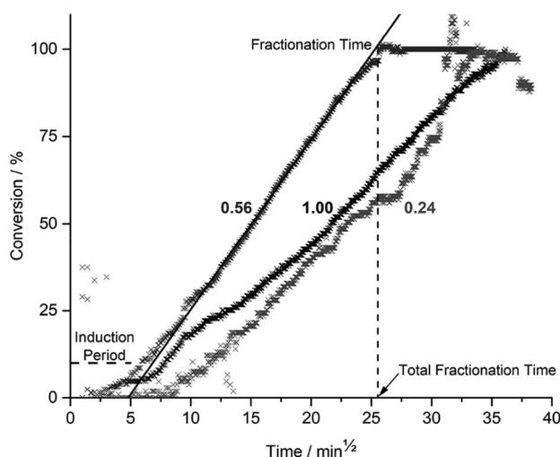
Fig. 2 Clear cast CYS<sub>5</sub> in 0.24 (light grey), 0.56 (dark grey), and 1.00 (black)  $x_{AA}$  at  $70\text{ }^\circ\text{C}$  as a function of square root time. The horizontal dashed line indicates the induction period, the solid line fitted from 25% to 75% conversion is used to calculate the fractionation rate, and the vertical dashed line indicates the total fractionation time.
