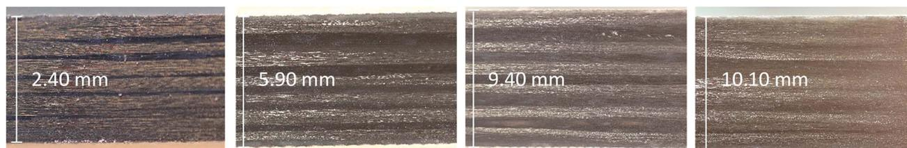
Fig. 5 Optical microscope cross-sectional pictures of the composite sandwich structures are shown, and from left to right are 1<sup>st</sup> to 4<sup>th</sup> infused composite, respectively.
