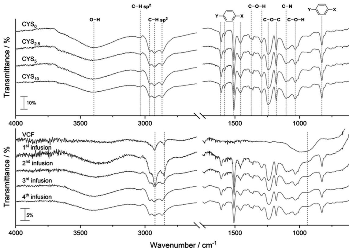
Fig. 1 FTIR spectra of the pure epoxy matrices (top) with peak assignments and spectra of the VCF together with the infused composites (bottom). The dashed lines indicate the VCF bands at  $960\text{ cm}^{-1}$ ,  $2852\text{ cm}^{-1}$ , and  $2932\text{ cm}^{-1}$ . All spectra except VCF are normalized by the peak found at  $828\text{ cm}^{-1}$ .
