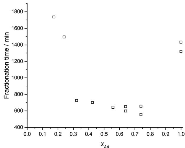
Fig. 3 CYS<sub>5</sub> total fractionation time at  $70\text{ }^\circ\text{C}$  in various  $x_{AA}$ .
