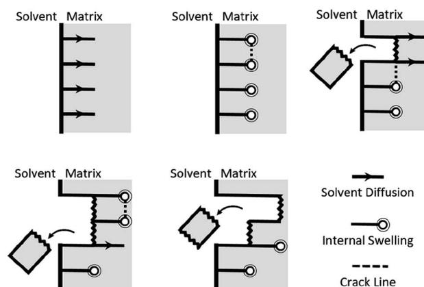
Fig. 8 Schematics of the proposed fractionation process.
