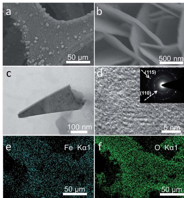
**Fig. 2** (a and b) SEM images for  $\text{Fe}_5\text{O}_7(\text{OH}) \cdot 4\text{H}_2\text{O}/\text{NF}$ . (c) TEM image of one single  $\text{Fe}_5\text{O}_7(\text{OH}) \cdot 4\text{H}_2\text{O}$  nanosheet. (d) HRTEM image and SAED pattern for the  $\text{Fe}_5\text{O}_7(\text{OH}) \cdot 4\text{H}_2\text{O}$  nanosheet. EDX elemental mapping images of (e) Fe and (f) O.
