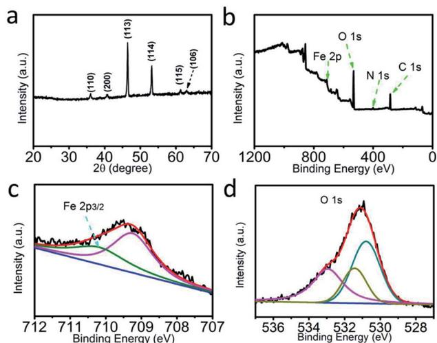
**Fig. 1** (a) XRD pattern of  $\text{Fe}_5\text{O}_7(\text{OH}) \cdot 4\text{H}_2\text{O}$ . (b) XPS survey spectrum of  $\text{Fe}_5\text{O}_7(\text{OH}) \cdot 4\text{H}_2\text{O}$ . XPS spectra of  $\text{Fe}_5\text{O}_7(\text{OH}) \cdot 4\text{H}_2\text{O}$  in the (c) Fe 2p and (d) O 1s regions.
