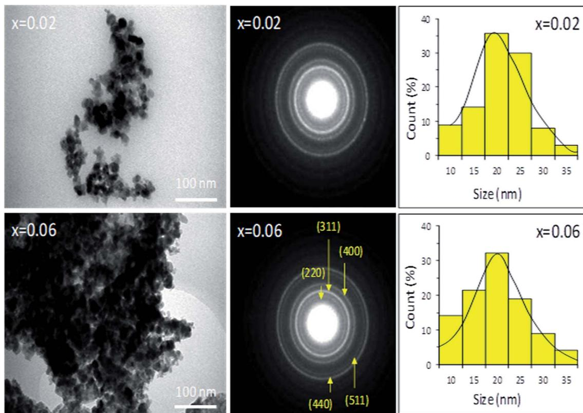
Fig. 4 TEM images, SAED patterns and size histograms of  $\text{Ni}_{0.4}\text{Cu}_{0.2}\text{Zn}_{0.4}\text{La}_x\text{Y}_x\text{Fe}_{2-x}\text{O}_4$  ( $x = 0.00 - 0.10$ ) NSFs for  $x = 0.02$  and  $0.06$  compositions.
