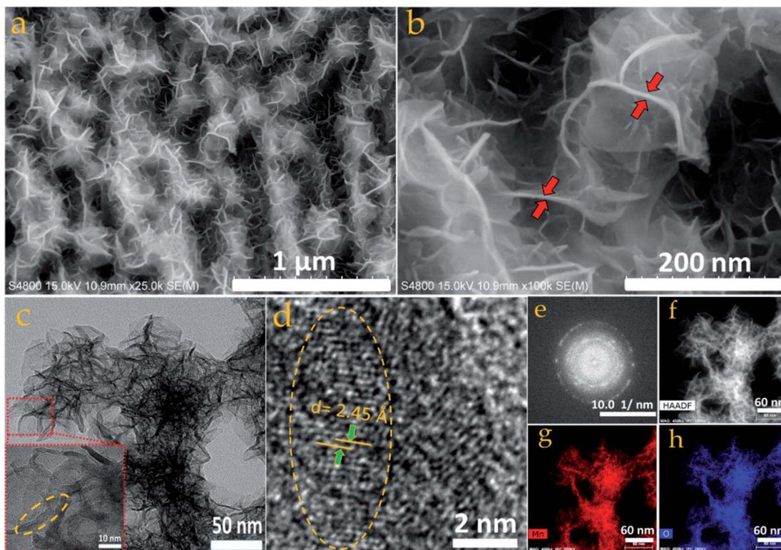
Fig. 4 (a) Low magnification and (b) high magnification FESEM image of  $\text{MnO}_2$  nanostructure featuring nanoflower-like morphology, and the corresponding (c) TEM (inset: HRTEM featuring porous structure and multilayer nano petals) and (d) HRTEM image with lattice fringes. (e) SAED pattern from the imaging area shown in (c). (f) HAADF image. (g and h) EDS mapping showing the presence of Mn and O elements.
