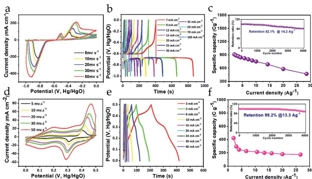
Fig. 5 (a and d) CV, (b and e) GCD, and (c and f) rate capability (with the insets) of the  $\text{Bi}_2\text{O}_3$  negatropde and  $\text{MnO}_2$  positrode in the first row and second row, respectively.
