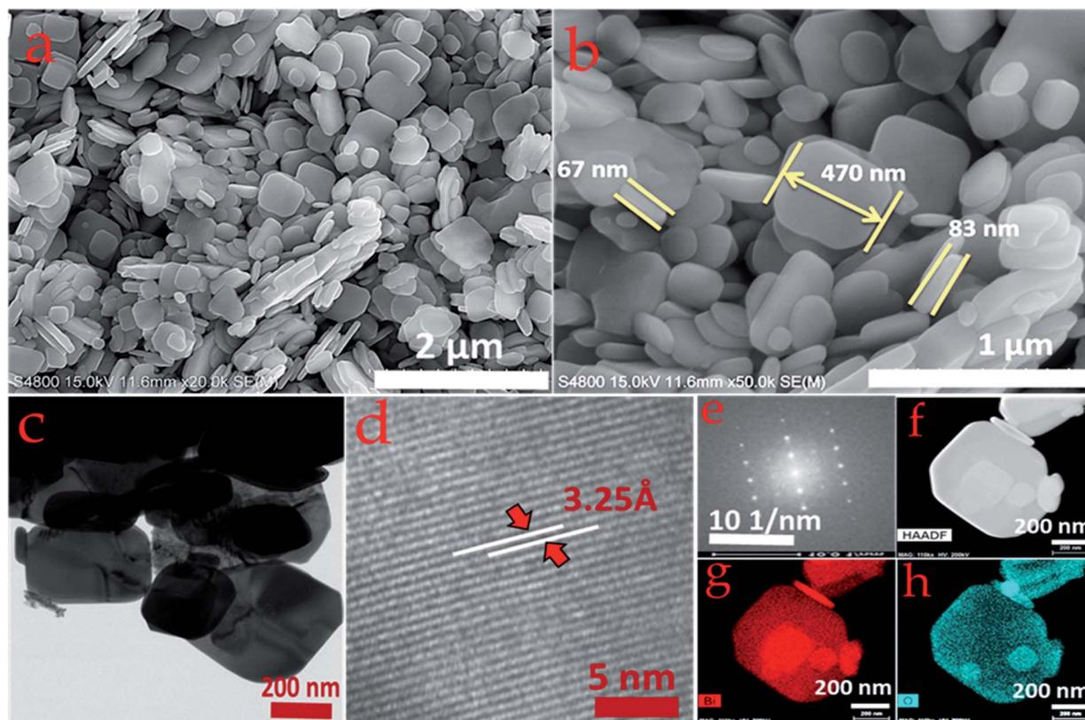
Fig. 3 (a) Low magnification and (b) high magnification FESEM images of the  $\text{Bi}_2\text{O}_3$  nanostructure and the corresponding (c) TEM and (d) HRTEM images. (e) SAED pattern. (f) HAADF image. (g and h) EDX mapping of Bi and O elements.
