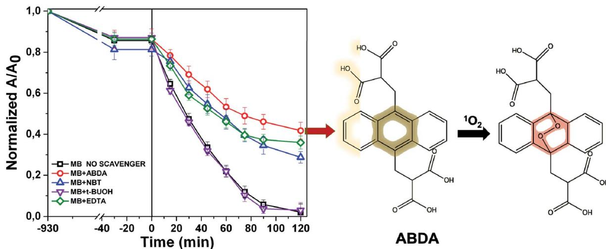
Fig. 11 Effect of ABDA, NBT, EDTA and *t*-BuOH radical-hole scavengers on the degradation rate of MB by using the Ni-free/G-Porph rings sample. The inhibition of the MB degradation due to the ABDA oxidation indicates the effective ROS production during 120 minutes of irradiation time. Among the produced ROS,  ${}^1O_2$  constitutes the predominant species.
