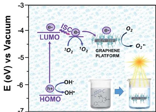
Fig. 12 Energy diagram of the proposed mechanism for the photocatalytic degradation of MB by using Ni-free/G-Porph rings as organic photosensitizer.
