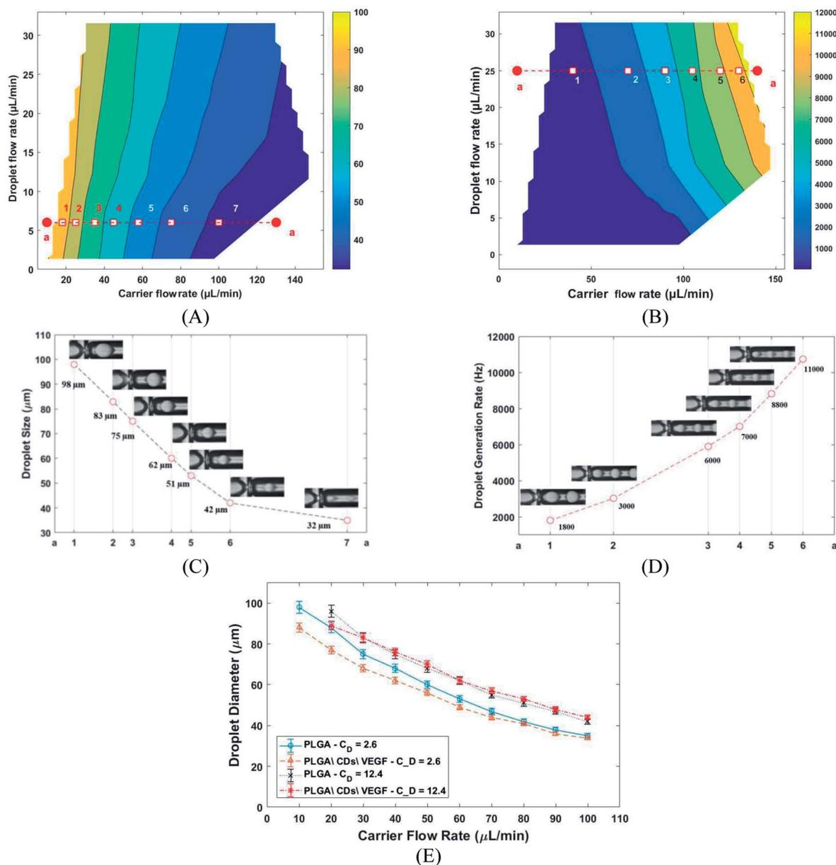
Fig. 4 (A) Droplet size, and (B) droplet generation rate for different values of carrier and droplet flow rate. (C) Droplet size formation in chip at  $C_d = 6.2 \mu\text{L min}^{-1}$  with different values of carrier flow rate, and (D) droplet generation rate at  $C_d = 25.2 \mu\text{L min}^{-1}$  with different values of carrier flow rate. (E) Droplet size variation against carrier flow for two different droplet flow includes PLGA/CDs/VEGF and PLGA as control.
