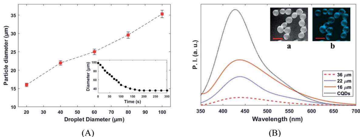
Fig. 6 (A) VEGF-loaded PLGA MPs sizes as a function of droplet size. The insets: size reduction profile of a tracked droplet as a function of time ( $C_f = 10 \mu\text{L min}^{-1}$ ,  $C_d = 2.5 \mu\text{L min}^{-1}$ ). (B) Photoluminescence response of VEGF-loaded PLGA MPs with different size (excitation wavelength 400 nm). The insets: fluorescence microscope image of VEGF-loaded PLGA MPs (22  $\mu$ m) (a): bright field and, (b): fluorescence (400 nm), (scale bar = 50  $\mu$ m).
