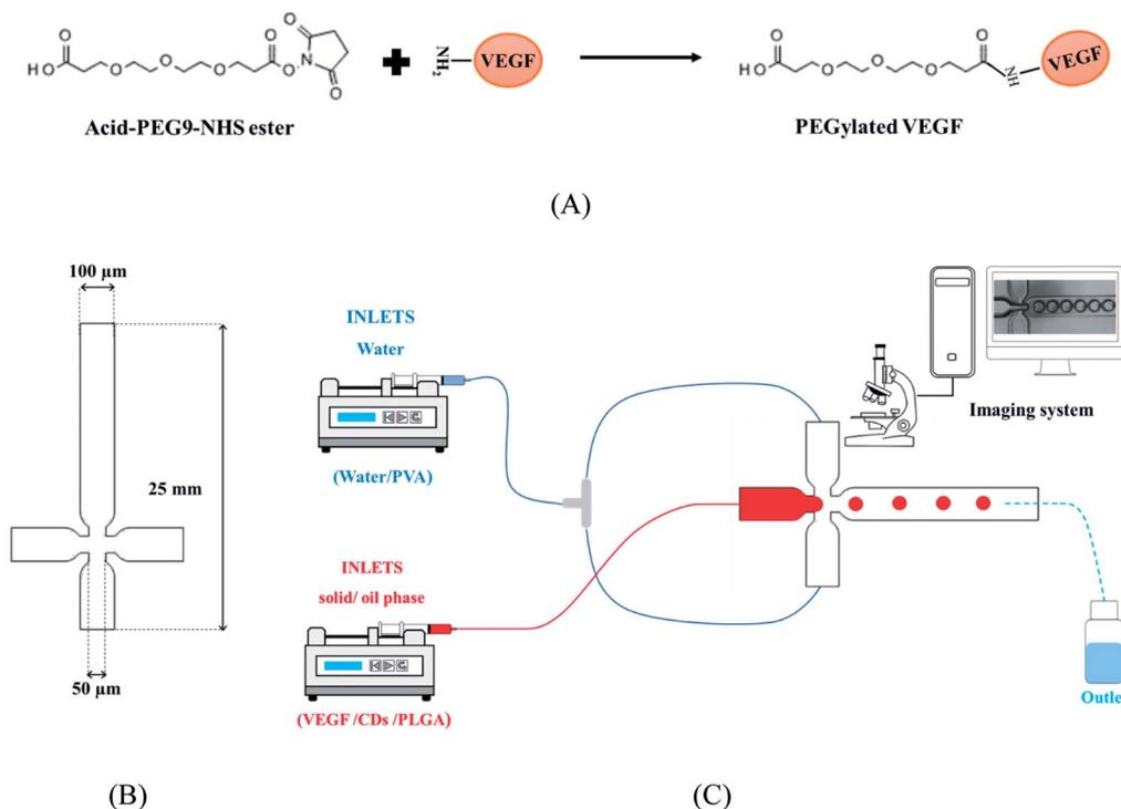
Fig. 1 (A) Illustration of VEGF PEGylation. (B) X-junction microfluidic chip designed, and (C) microfluidic set up for VEGF-loaded MPs production.
