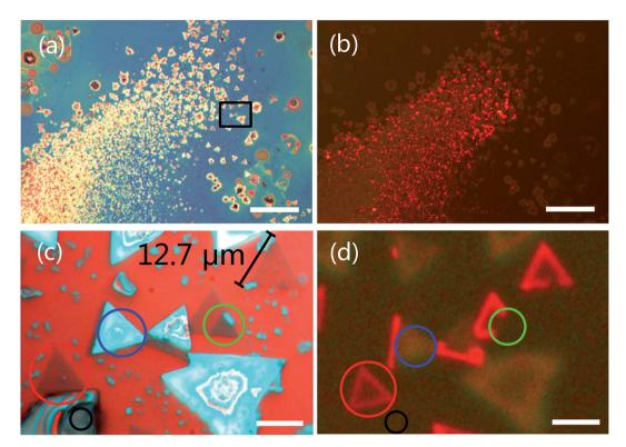
Fig. 2 Optical microscopy (a) and photoluminescence (PL) (b) images of  $WS_2$  layers grown on  $SiO_2/Si$  substrate. (c) Magnified optical microscopy and corresponding PL images taken from the boxed area in (a). (a) and (b) were taken at same location. The scale bars in figure (a) and (b) represent 100  $\mu$ m, and 10  $\mu$ m in (c) and (d). The red color in (b) and (d) is due to the PL emission of monolayer  $WS_2$ .
