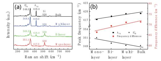
Fig. 3 (a) Raman spectra of monolayer (red line), bilayer (green line), multilayer (blue line) and bulk (black line) WS<sub>2</sub> corresponding to the sample in Fig. 2c. (b) Thickness dependent of Raman peak position and the peak frequency difference between  $E_{2q}^1$  and  $A_{1q}$ .
