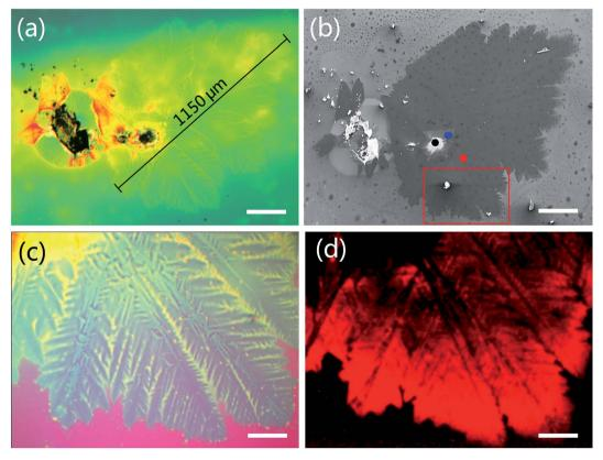
Fig. 5 Optical microscopy (a) and SEM (b) images of  $WS_2$  film taken at the same location. (c) Magnified optical microscopy image of (a). (d) The photoluminescence (PL) image corresponding to the sample of (c). (c) and (d) are taken at the same location. The red color in (d) is due to the PL emission of monolayer  $WS_2$ . The scale bars in figure (a), (b), (c) and (d) represent 200  $\mu$ m, 200  $\mu$ m, 50  $\mu$ m and 50  $\mu$ m, respectively.
