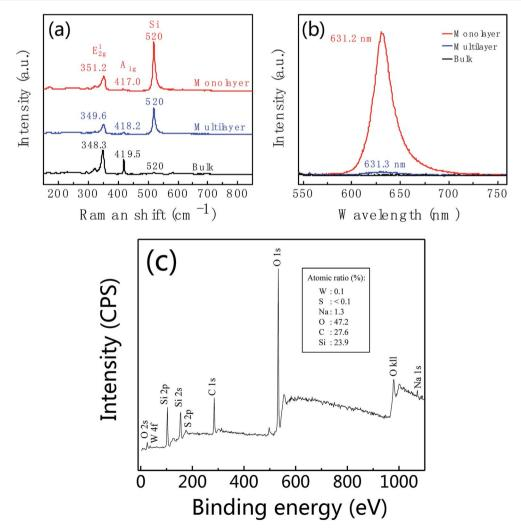
Fig. 6 Raman (a) and photoluminescence (b) spectra of  $WS_2$  taken from the regions marked with red, blue and black spots in Fig. 5b. (c) XPS of leaf-like domain of as-prepared  $WS_2$ . Insert is atomic ratio.
