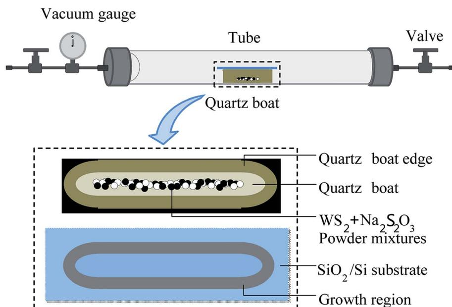
Fig. 1 Schematic diagram of monolayer WS<sub>2</sub> growth setup (upper), quartz boat and precursor (middle) and growth region (bottom) on SiO<sub>2</sub>/Si substrate. Growth zone shape is consistent with the edge of the quartz boat.
