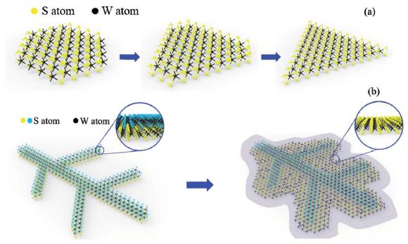
Fig. 7 Schematic drawing of the growth mechanism of (a) triangular WS<sub>2</sub> and (b) leaf-like WS<sub>2</sub>.
