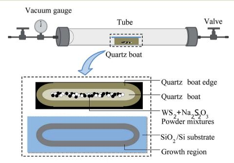
Fig. 1 Schematic diagram of monolayer WS<sub>2</sub> growth setup (upper), quartz boat and precursor (middle) and growth region (bottom) on SiO<sub>2</sub>/Si substrate. Growth zone shape is consistent with the edge of the guartz boat.
