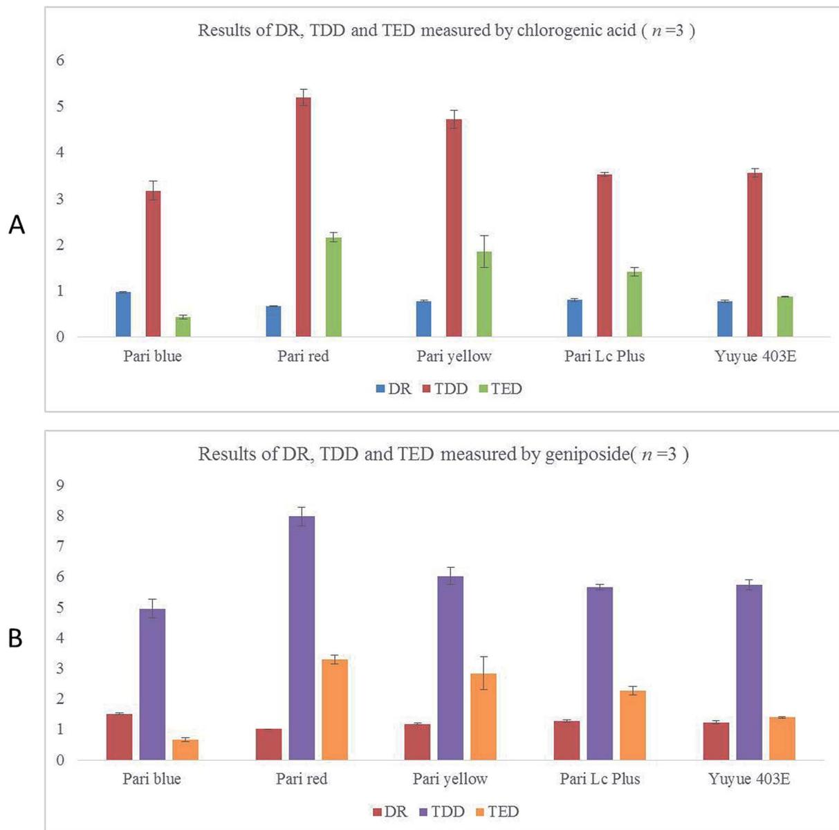
Fig. 3 Uniformity delivery dose results of five different nebulizers determined by HPLC. (A) Results measured by chlorogenic acid ( $n = 3$ ). (B) Results measured by geniposide ( $n = 3$ ). DR, TDD and TED represented delivery rate, total delivered dose and total exhalation dose, respectively.
