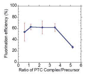
Fig. 3 Investigation of the effect of the phase transfer catalyst complex  $(K^+/K_{2,2,2})$  to precursor ratio.
