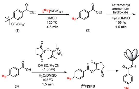
Fig. 1 Overall radiosynthetic scheme of [<sup>18</sup>F]SFB on the EWOD chip and the conjugation of the <sup>18</sup>F-labeled prosthetic group to the PSCA-diabody. The conjugation is performed in sodium-borate buffer (SBB, 50  $\mu\text{mol L}^{-1}$ , pH 8.7) and incubated for 10 min at 34  $^\circ\text{C}$ . Cartoon of diabody is not to scale.
