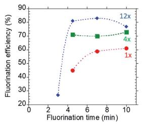
Fig. 4 Kinetics of the fluorination reaction at different reagent concentrations. Reactions were performed in 2  $\mu L$  of DMSO at 120 °C. The blue trace (diamond marker) represents the optimized concentration, i.e. 12× the concentration used in the macroscale reaction; the green trace (square marker) represents 4× concentrations and the red trace (circular marker) represents the same concentration as used in the macroscale.
