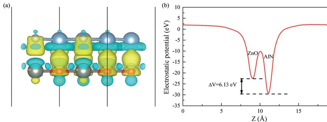
Fig. 6 (a) The charge density difference of the ZnO/AlN composite. Yellow and cyan regions separately represent charge accumulation and depletion. (b) The planar averaged electrostatic potential of the ZnO/AlN composite as a function of position in the vacuum direction.
