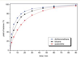
Fig. 3 The influence of the solvent for the model oxidation of 2-adamantanone. Reaction conditions: 2-adamantanone (0.100 g, 0.67 mmol), perdecanoic acid (1.34 mmol), solvent (2 mL), 25 °C, 1200 rpm.
