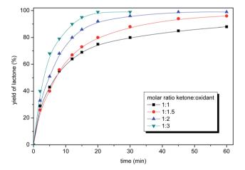
Fig. 5 The influence of molar ratio ketone : oxidant for the model oxidation of 2-adamantanone. Reaction conditions: 2-adamantanone (0.100 g, 0.67 mmol), perdecanoic acid, toluene (2 mL), 35  $^{\circ}$ C, 1200 rpm.
