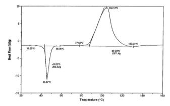
DSC of perdecanoic acid at a heating rate of 10 °C min<sup>-1</sup>.
