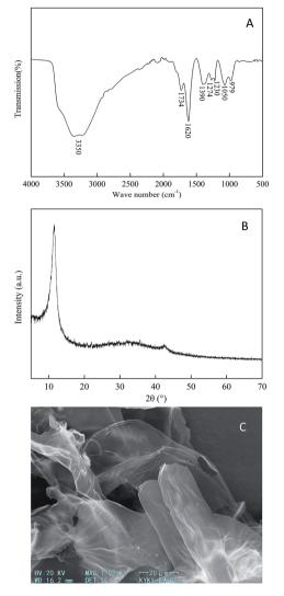
Fig. 2 (A) FT-IR spectrum (B) XRD pattern and (C) SEM image of the as-prepared GO.
