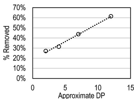
Fig. 3 Impact of DP on model oligosaccharide removal by hydrophobic resin (3 mg ml<sup>-1</sup> starting concentration).
