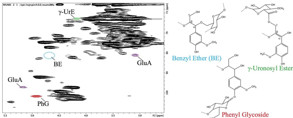
**Fig. 1** 2D-HSQC NMR spectrum of hydrophobic adsorbate from *Miscanthus* autohydrolysate showing the presence of cross-correlated peaks associated with uronosyl ester and phenyl glycosidic LCC linkages.
