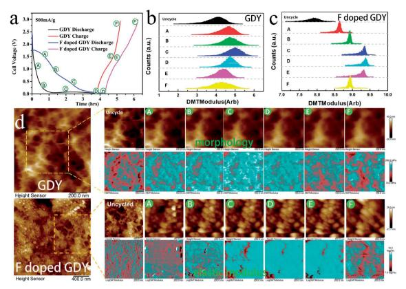
Fig. 5 (a) Galvanostatic cycling of GDY and F doped GDY at 500 mA  $g^{-1}$ . A to D correspond to the intercalation process and D to F correspond to the deintercalation process. Area statistics of elastic modulus variations in different states during discharge/charge of (b) GDY and (c) F doped GDY. (d) *In situ* Kelvin probe atomic force microscope record of morphology and elastic modulus phase in different chemical states during discharge/charge.
