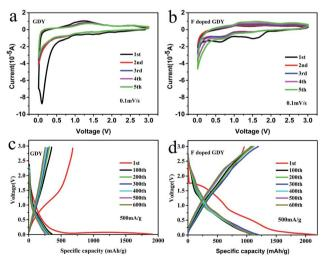
Fig. 3 (a and b) Cyclic voltammetry curves of the GDY and F doped GDY based electrode, scan rate is 0.1 mV s $^{-1}$ . (c and d) Galvanostatic charge/discharge profiles of GDY and F doped GDY electrodes at a current density 500 mA  $\rm g^{-1}$ , recorded between 0.01 mV and 3 V.
