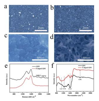
Fig. 1 (a) SEM image morphology of GDY film grown on the surface of copper foil. (b) SEM morphology of the F doped GDY film. Highmagnification SEM of (c) GDY and (d) F doped GDY. (e) Raman spectra of GDY and F doped GDY. (f) FTIR spectra of GDY and F doped GDY film on copper foil.
