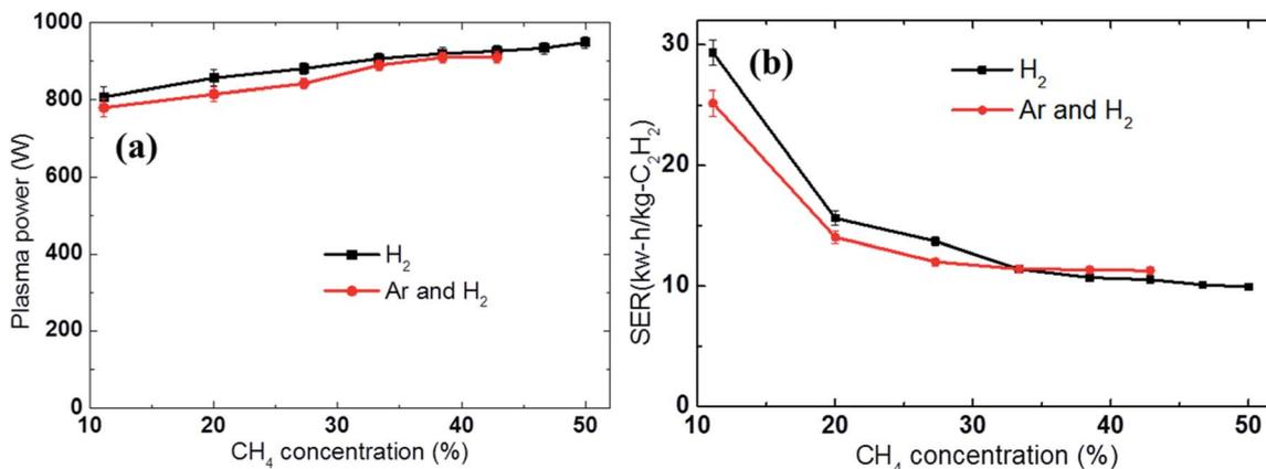
Fig. 4 Effect of the methane feed rate on the (a) plasma power and (b) energy cost (SER) using either H<sub>2</sub> (8 SLPM) or an Ar and H<sub>2</sub> mixture (4 SLPM of Ar and 4 SLPM of H<sub>2</sub>) as the discharge gas.
