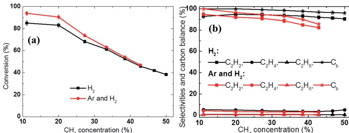
Fig. 5 Effect of the methane feed rate on the (a) conversion and (b) selectivity and carbon balance using either H<sub>2</sub> (8 SLPM) or an Ar and H<sub>2</sub> mixture (4 SLPM of Ar and 4 SLPM of H<sub>2</sub>) as the discharge gas.
