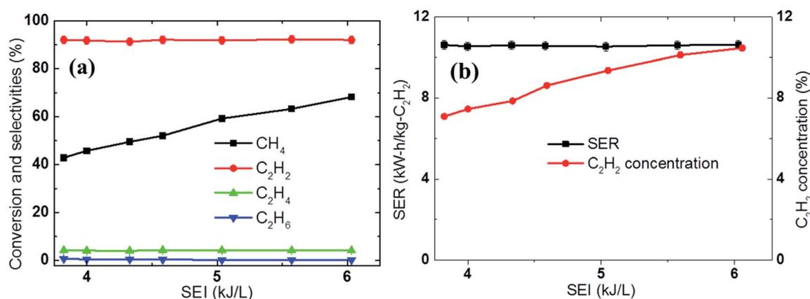
Fig. 6 Effect of the SEI on the (a) conversion, selectivity, and carbon balance and (b) SER and C<sub>2</sub>H<sub>2</sub> concentration using CH<sub>4</sub> (6 SLPM) and H<sub>2</sub> (8 SLPM).
