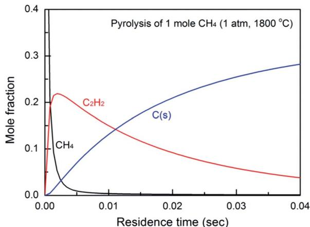
Fig. 1 Effect of residence time (reaction time) on the product yield, calculated based on a simplified reaction model proposed by Holmen.<sup>38</sup>
