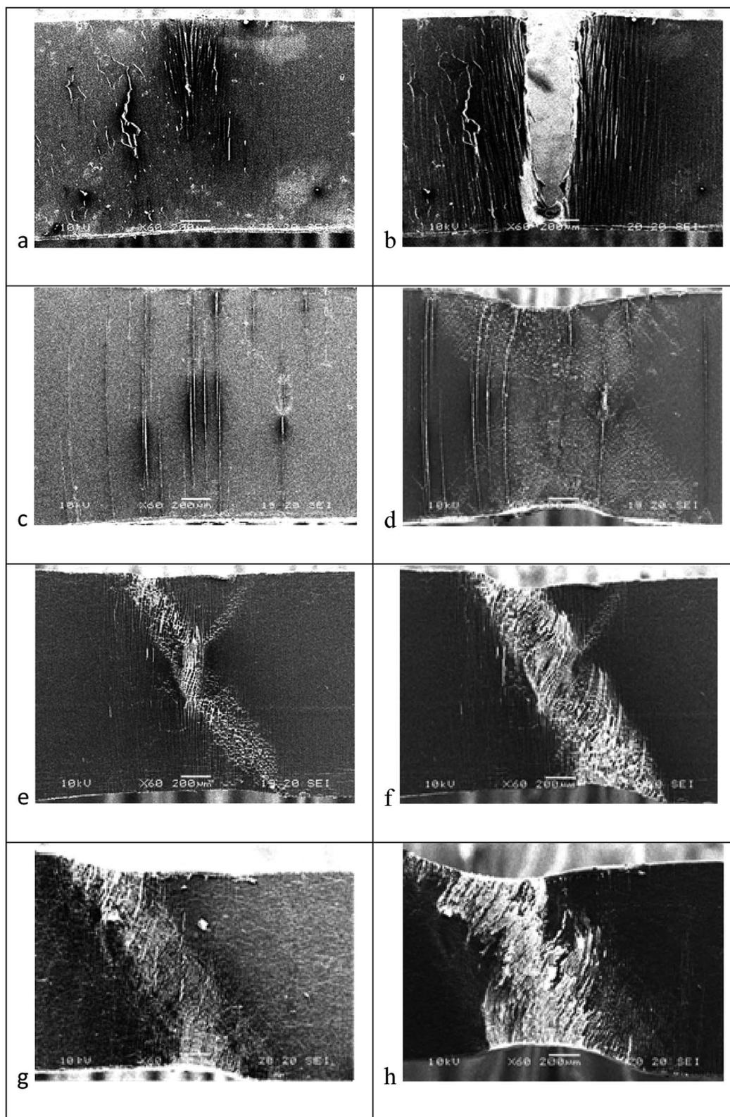
Fig. 4 *In situ* SEM micrographs of the structure evolution of: PLA/PBAT (97/3) blend (a and b), PLA/PBASGT (90/10) blend (c and d), PLA/PBASGT (97/3) composite (e and f), and PLA/PBAT (90/10) composite (g and h) subjected to tensile test. The respective deformations are 0.071 (a), 0.077 (b), 0.140 (c), 0.262 (d), 0.104 (e), 0.182 (f), 0.166 (g), and 0.322 (h).
