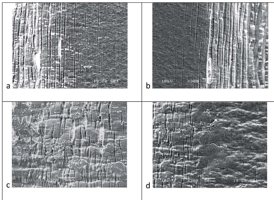
Fig. 6 SEM micrographs showing the processes of localization and thickening of: crazes in PLA/PBASGT (97/3) composite (a) and PLA/PBAT (97/3) (b) composite, and microcracks in PLA/PBASGT (90/10) composite in vicinity of neck (c) and far away from neck (d).
