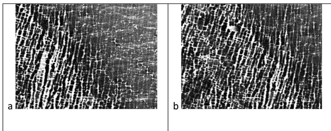
Fig. 7 SEM micrographs showing the development of a shear band in PLA/PBASGT (90/10) composite. The respective deformations are 0.250 (a), 0.300 (b).
